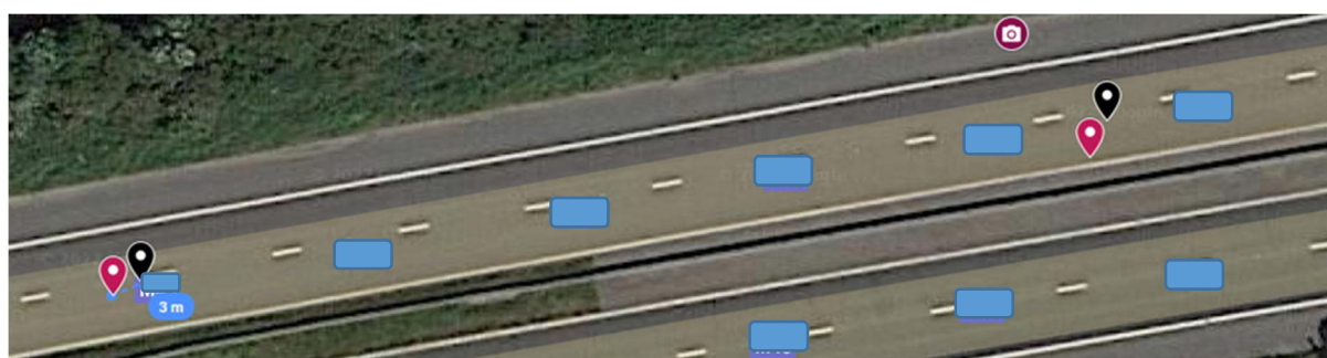
Figure 14: Position of Radar ClearWay (Red) vs GPS (black) stops (blue boxes used to hide distinguishing information)
