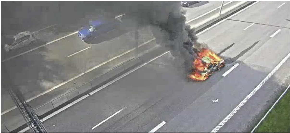
Figure 25: Stopped vehicle in live lane in Sweden Motorway, detected by the Navtech Radar Clearway system
