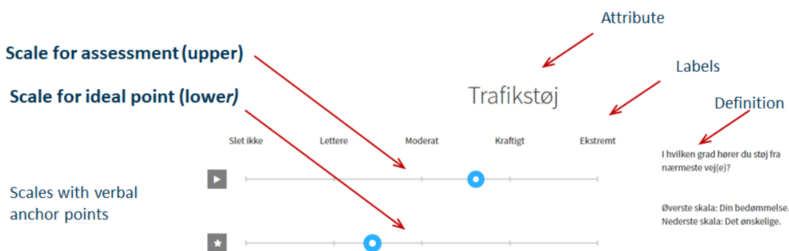
Figure 83: Example on answering scales according to the Ideal profile method for the sound walk. This example is for the assessment of traffic noise. For other attributes, definitions, and scale labels (translated to English), see Table 6. In the data processing the position of the sliders are measured on a 0-100 scale.
