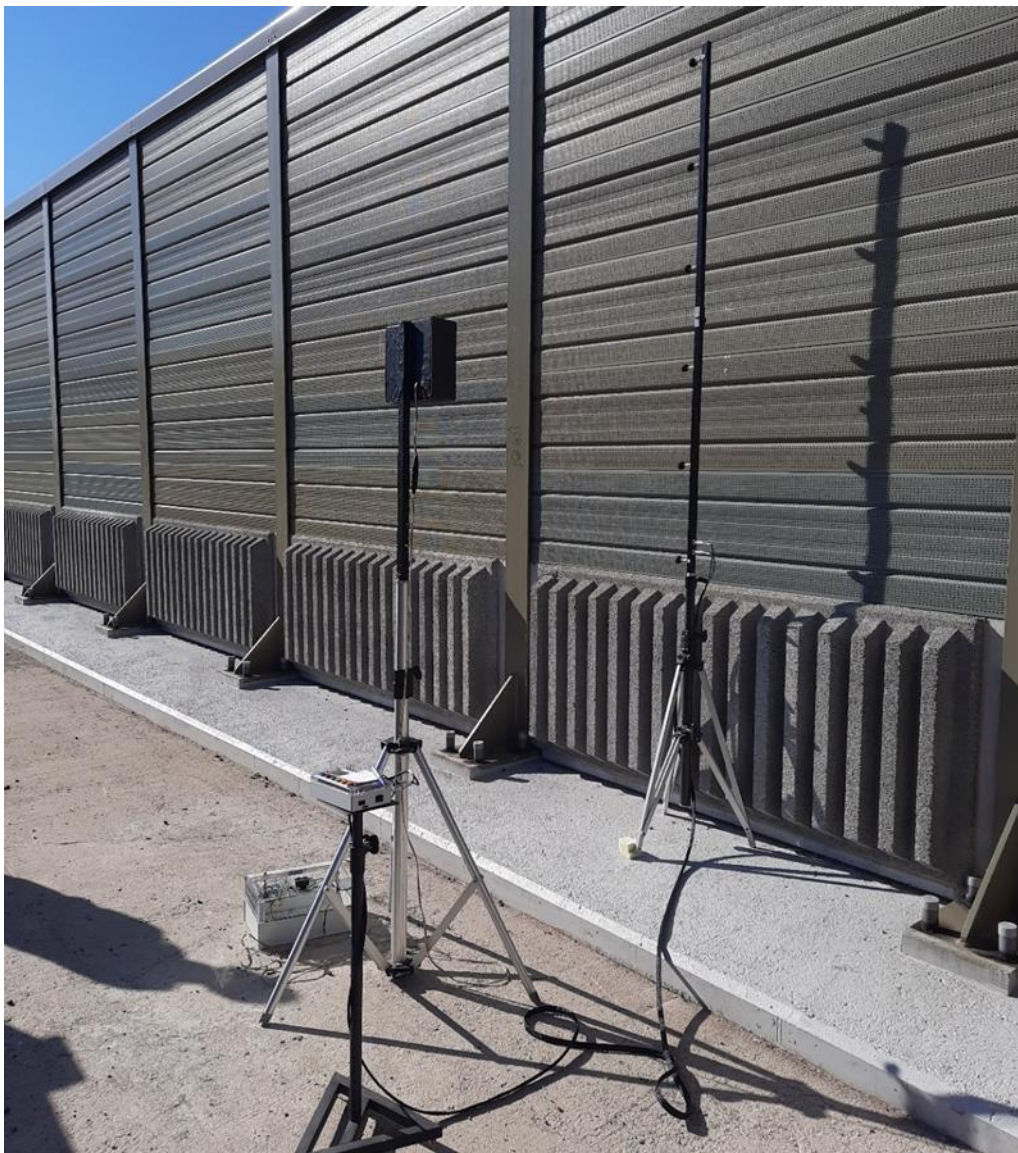
Figure 17. Microphone antenna, loudspeaker and control device in place for the quick sound reflection index measurements.
