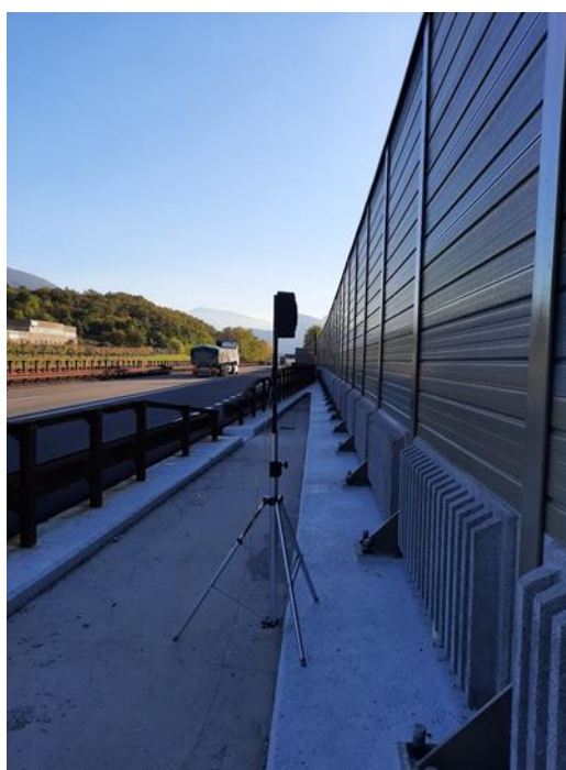
Figure 23. Loudspeaker in place for the quick sound insulation index measurements.
