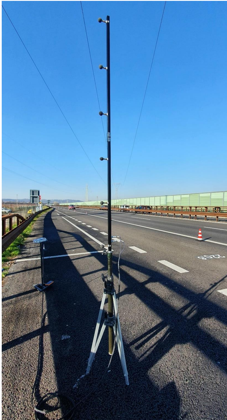
Figure 16. The linear microphone antenna on a supporting stand. The microphones are labelled "M1" to "M6" from the bottom to the top. On a flat ground, M1 is at 1,20 m from the ground. The spacing between subsequent microphones is 0,40 m.
