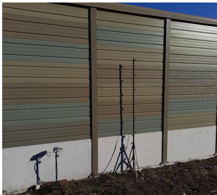
Figure 22. Microphone antenna and control device in place for the quick sound insulation index measurements.
