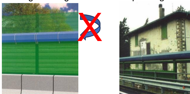
Figure 30: Use added devices carefully as they may not protect above the shadow line
