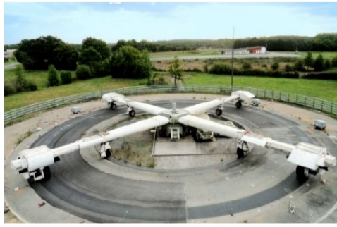
Figure 4: (a) IFSTTAR accelerated pavement test facility and (b) Comparison of pavement deflection between deflectometer, geophone and accelerometer after Bahrani et al. (2020)
