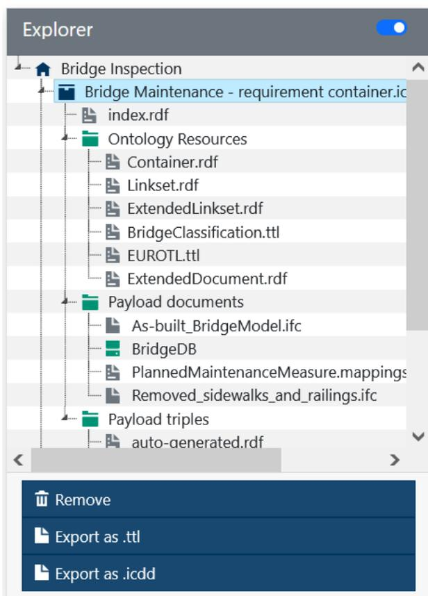
Figure 10: Explorer with the options to remove and export containers
