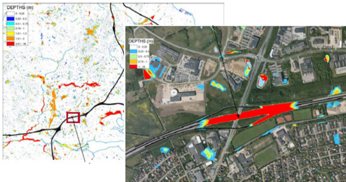
Figure 2. Identified Blue spots (Level 1) showing their area, volume and depth (example from ROADAPT case study Öresund).
