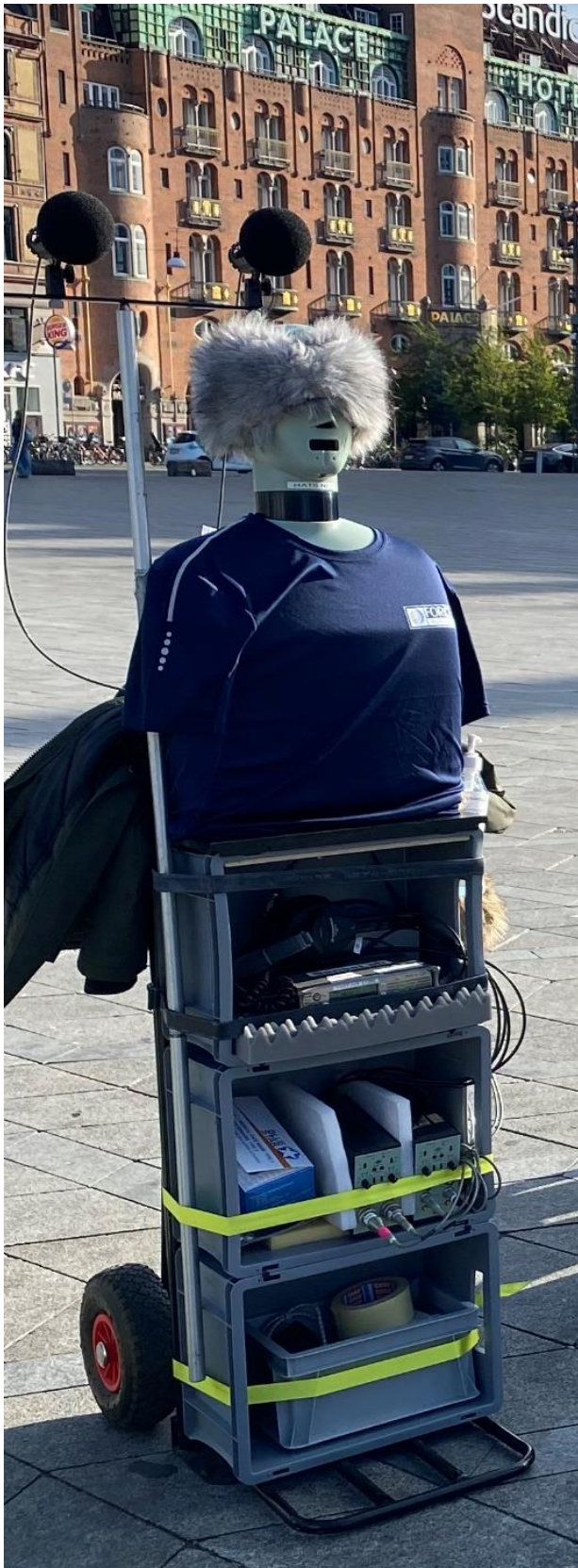
Figure 84: The portable equipment for the sound recordings. The “hair” on the HATS is a windscreen.
