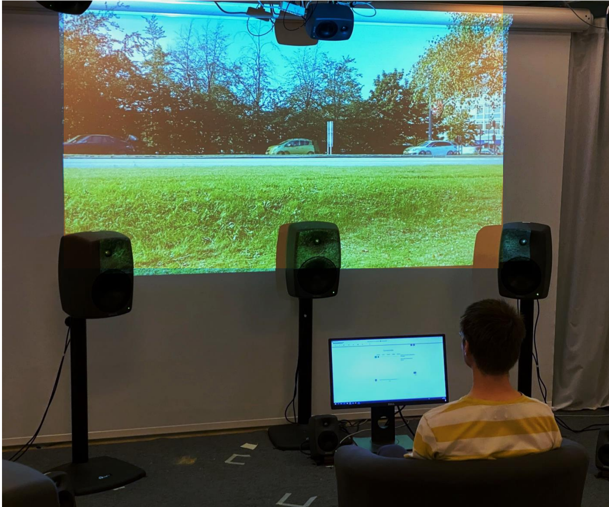
Figure 32: The SenseLab listening room at FORCE Technology. The sound is played from the stereo setup and the video is shown at the large screen. The projector for the video is outside the listening room. The PC-screen is for the user interface.
