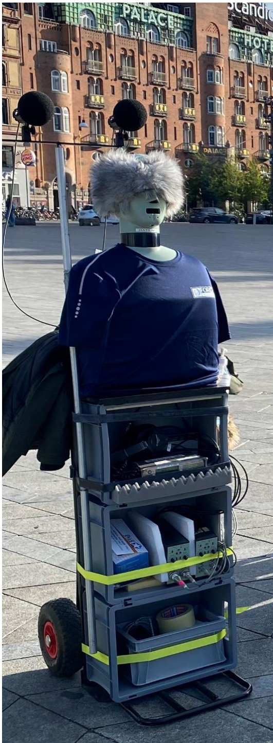
Figure 9 The portable equipment for the sound recordings. The "hair" on the HATS is a windscreen.
