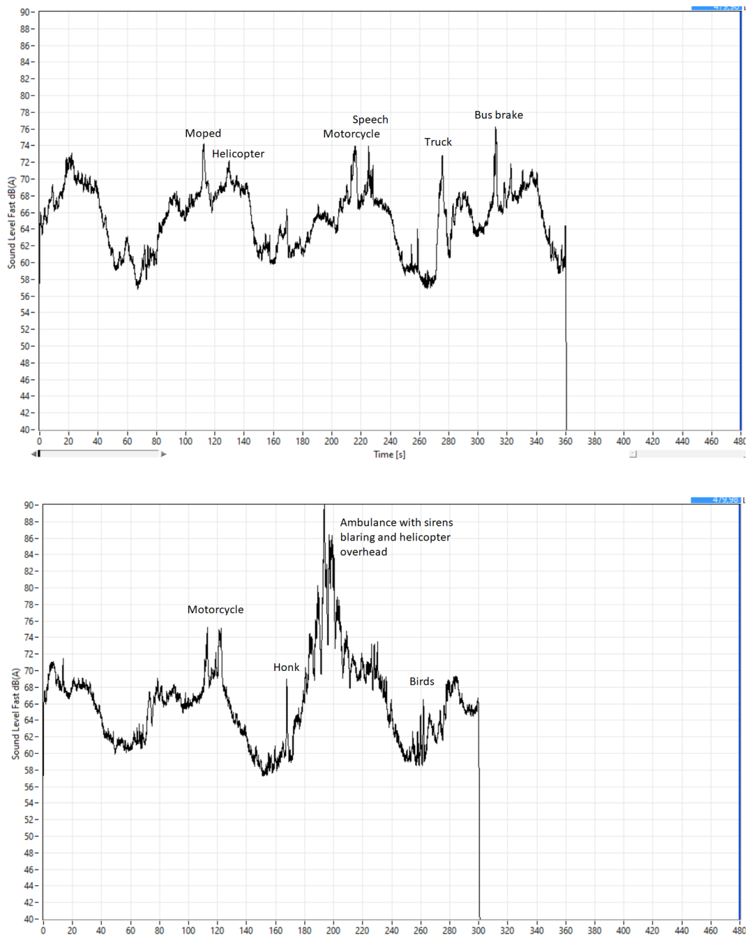
Figure 34 Position 2. Level recordings (A-weighted, F). Upper: Sound walk no. 3. Lower: Sound walk no. 4, 160-260 s excluded from analysis.
