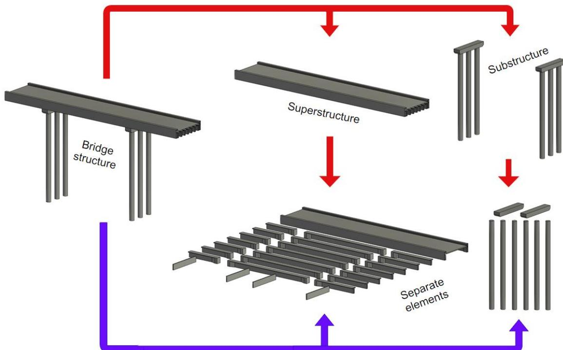
Figure 8: Different approaches of bridge structure decomposition used in different NRAs
