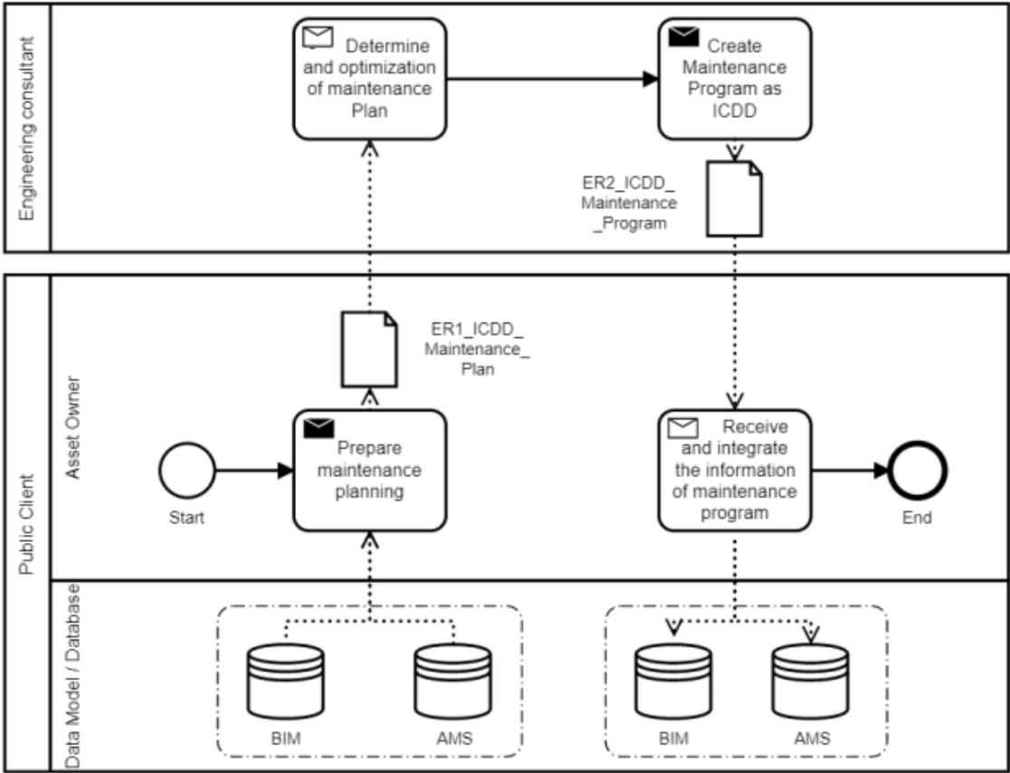
Figure 1: Data exchange for maintenance planning of roads
