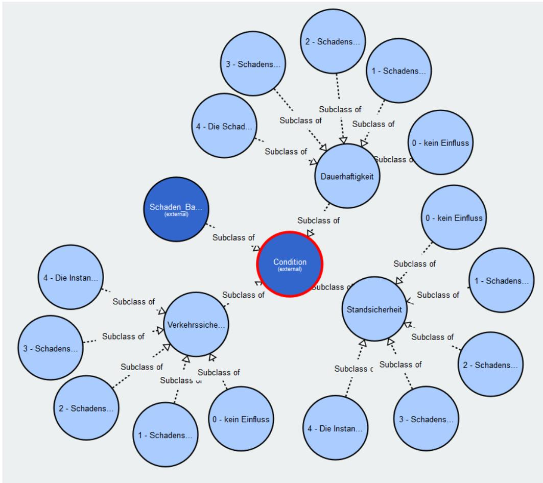
Figure 14: Condition assessment ontology according to ASB-Ing
