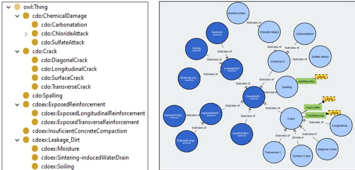
Figure 13: Concrete damage ontology (cdo)
