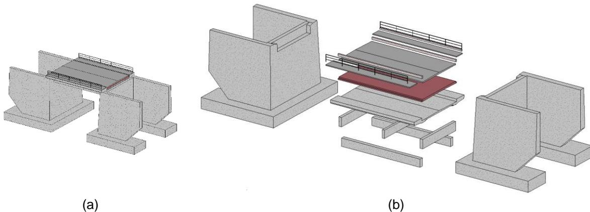
Figure 17: Original exemplary BrIM: (a) collapsed, and (b) exploded view
