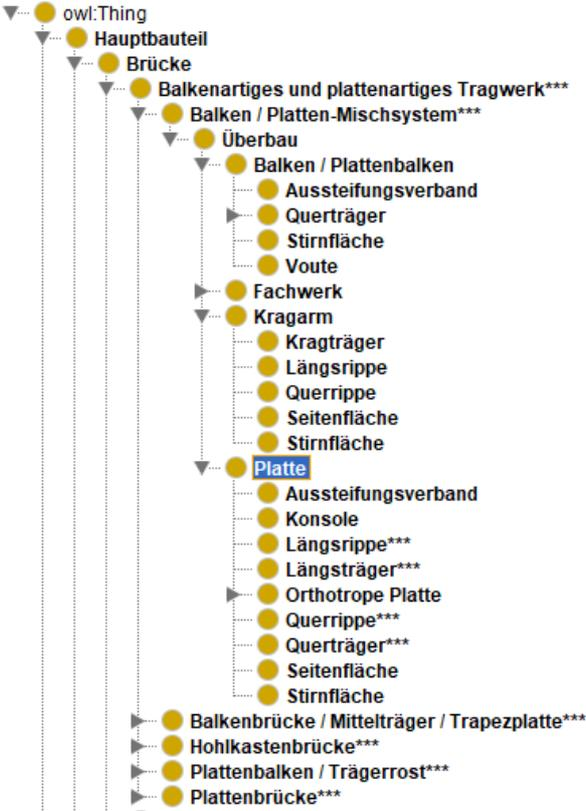
Figure 9: ASB-ING Classification ontology. Class hierarchy snippet showing bridge (beam/slab mixed system) superstructure (Brücke:Balken/Platten-Mischsystem:Überbau) classes.
