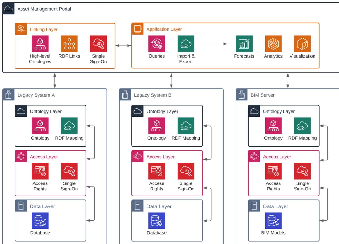
Figure 26: Reference architecture for BIM-based asset management
