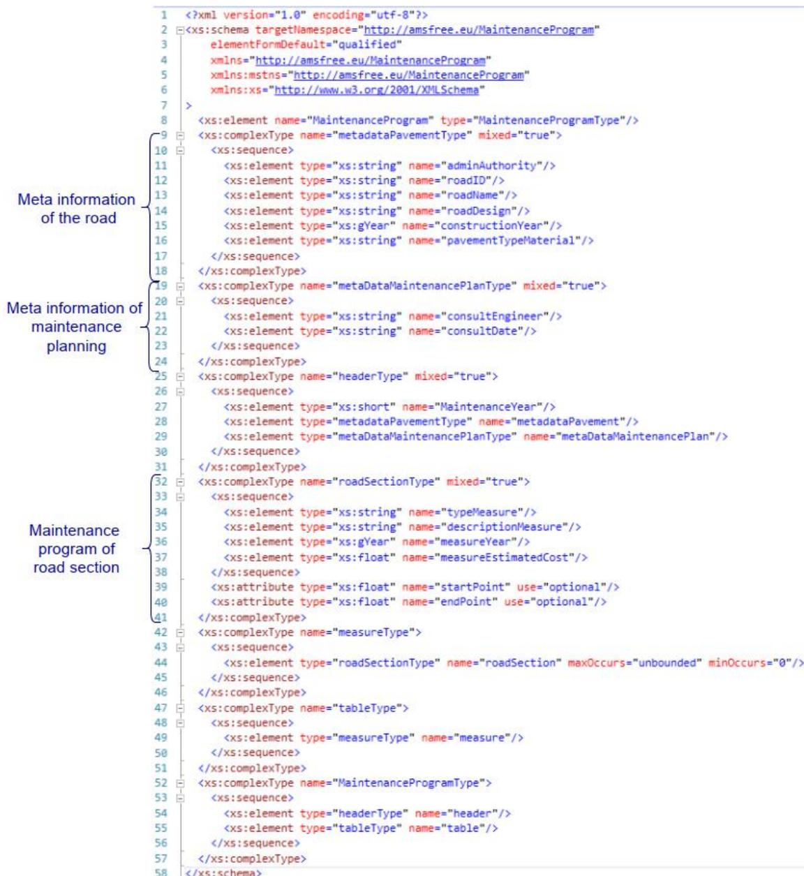
Figure 7: Maintenance program as XML schema
