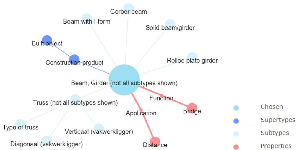
Figure 12: Bridge girder represented by the CB-NL ontology
