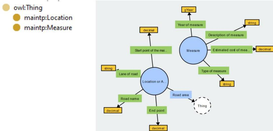
Figure 6: Maintenance program ontology (MAINTP)
