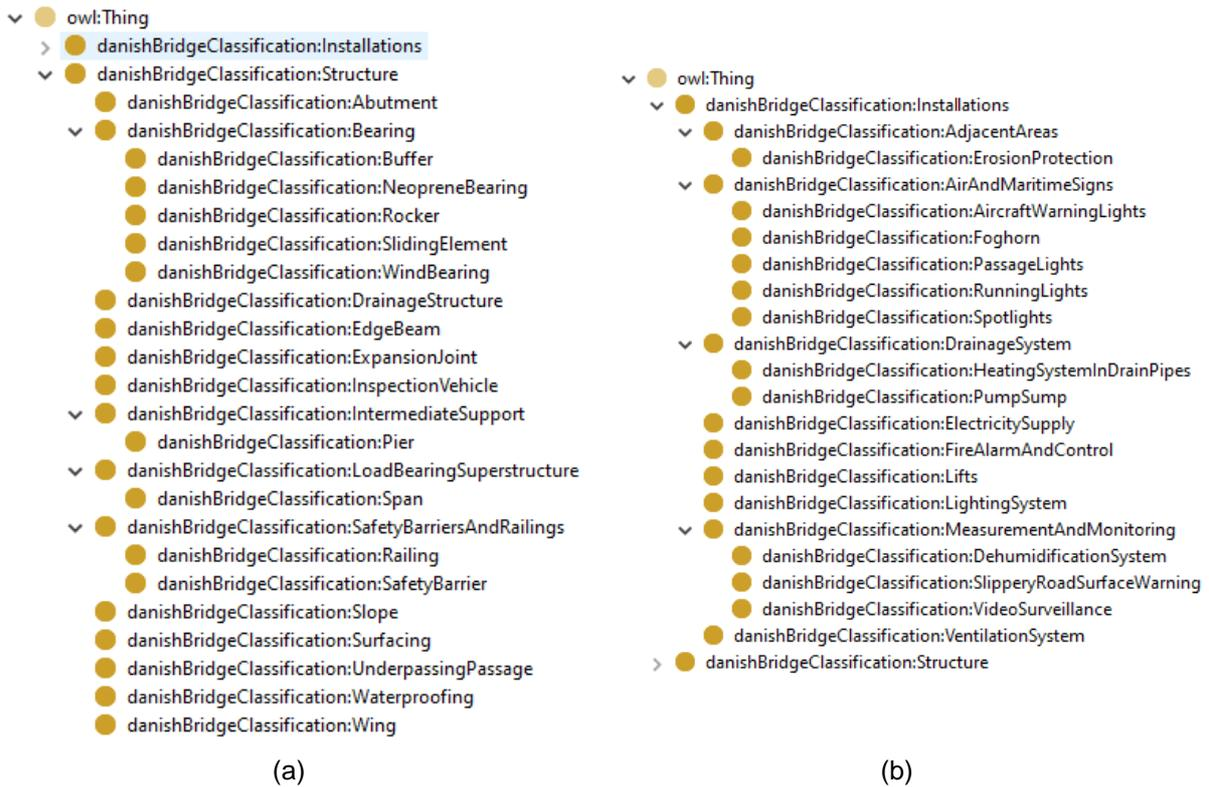
Figure 11: Class hierarchy of the Danish bridge classification ontology:
