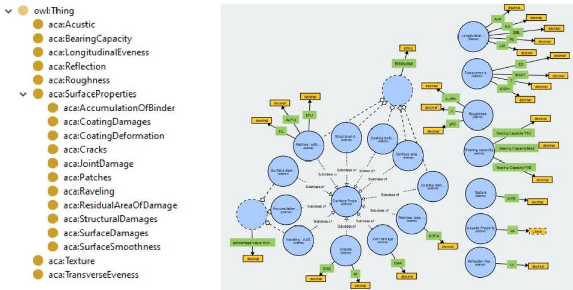
Figure 5: Asphalt condition assessment ontology (ACA)
