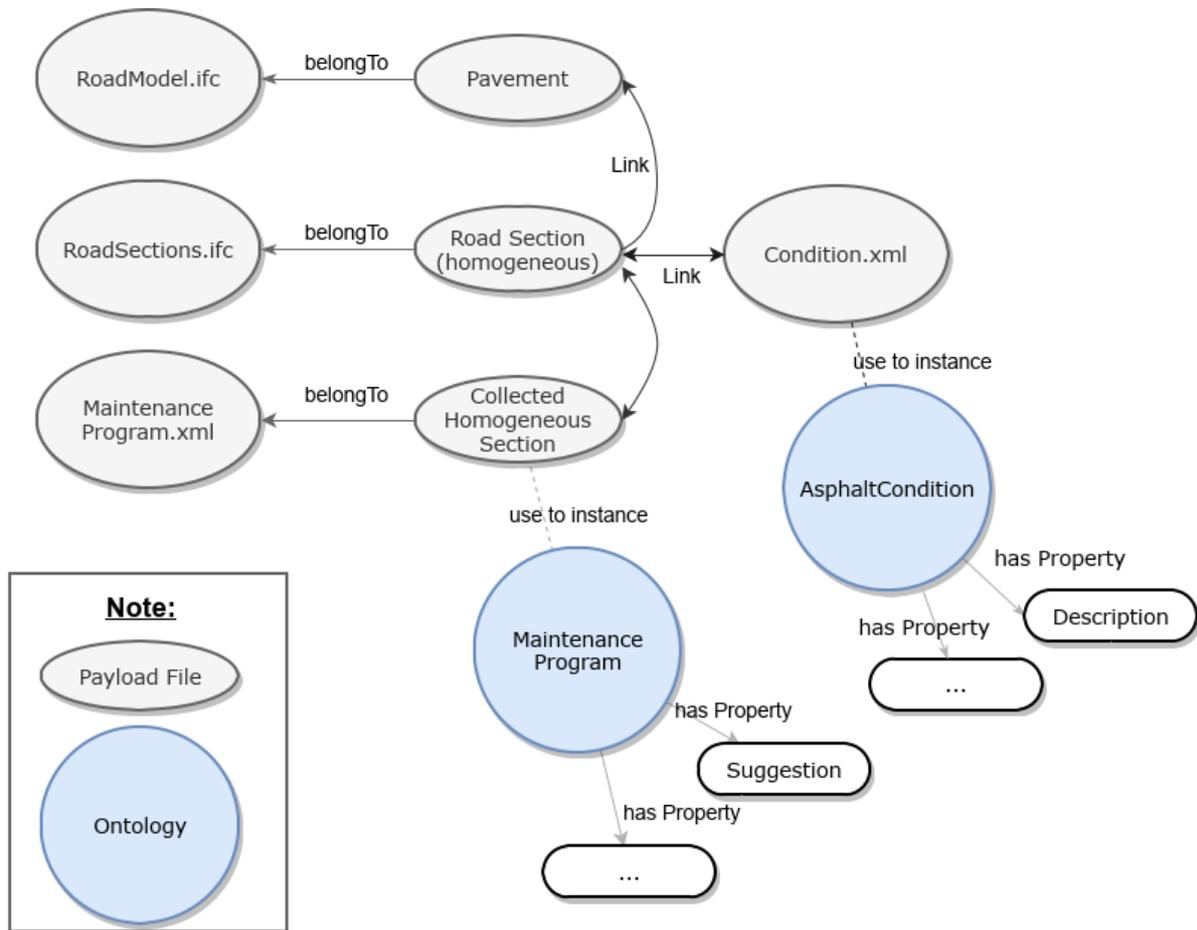
Figure 4: Relations of the information container for the maintenance planning of roads
