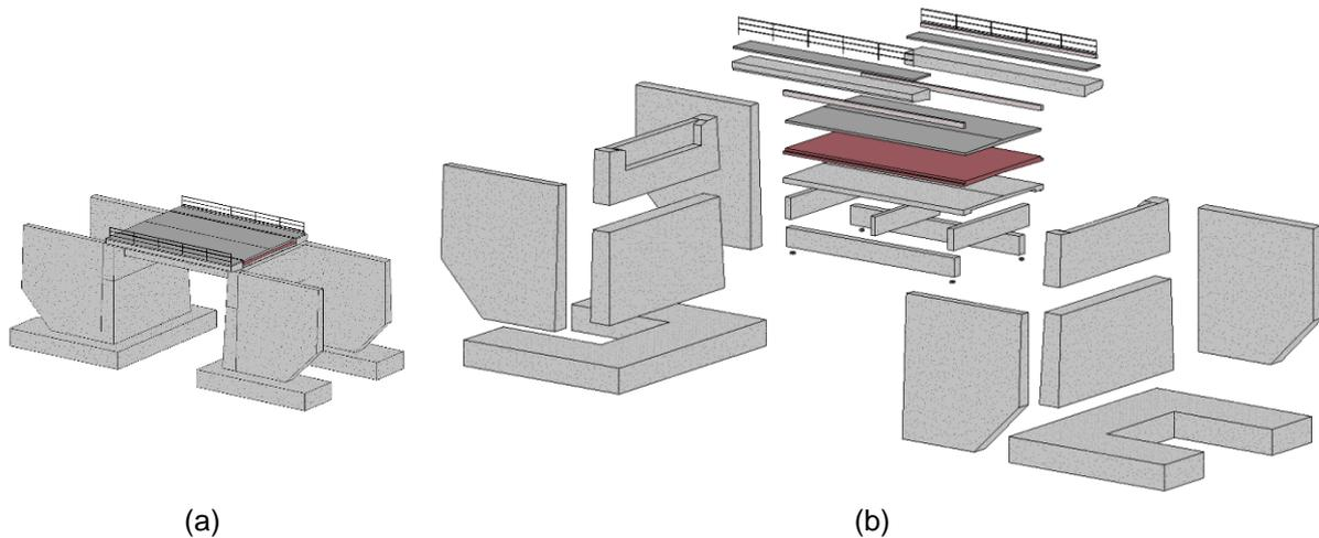
Figure 18: Remodelled exemplary BrIM: (a) collapsed, and (b) exploded view
