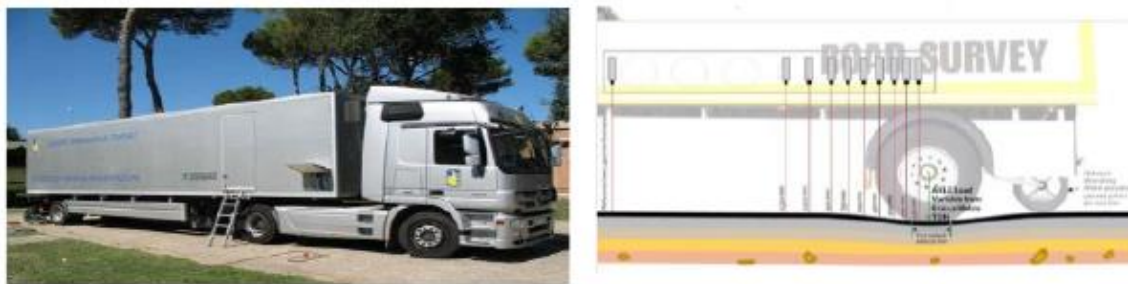
Figure 2 a) Traffic Speed Deflectometer (TSD) vehicle and b) the layout of its lasers, after Wright et al. 2016)
