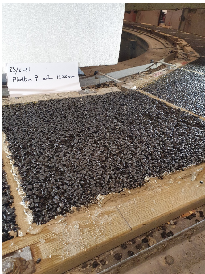
Figure 5-4. Stone losses after 12 000 laps at 30 °C for long term aged Fibra 4 mix.
