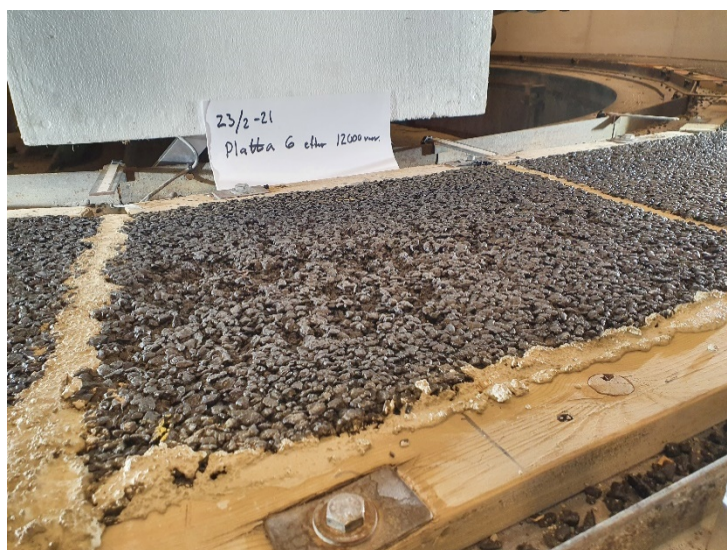
Figure 5-3. Stone losses after 12 000 laps at 30 °C for long term aged Fibra 3 mix.
