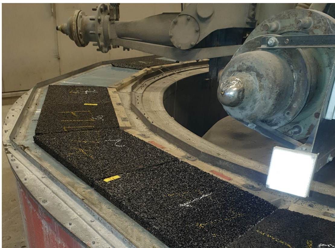
Figure 5-1. Laying of asphalt plates in the CRS.
