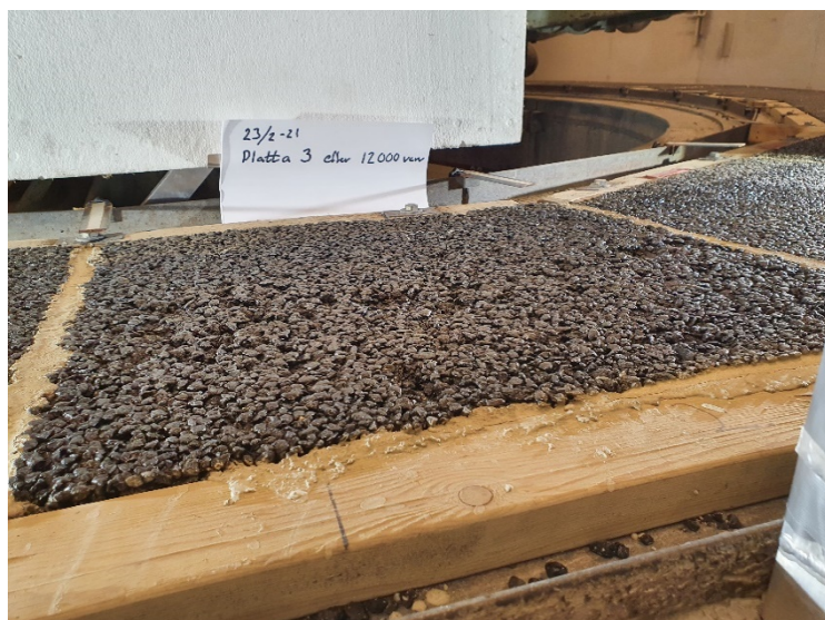
Figure 5-2. Stone losses after 12 000 laps at 30 °C for long term aged Fibra 1 mix.
