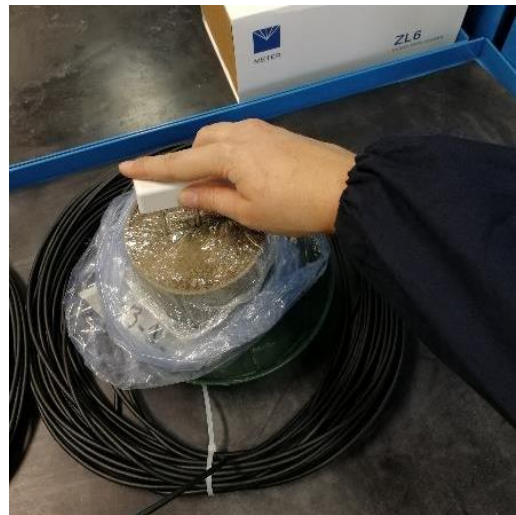
Figure C2. Preparation of the mortar specimens: a) mixing, b) Proctor compaction, c) specimen compacted, d) creation of the needles allocations, e) specimen ready for the installation of the sensor, f) installation of the sensor
