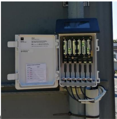
Figure 21. Sensors installation (phases F to J): a) sensors installed, b) sensors and cables, c) sensor covered by cold recycled mortar, d) cables blocked with cementitious mortar, e) data logger installation, f) sensors connected to the data logger.
