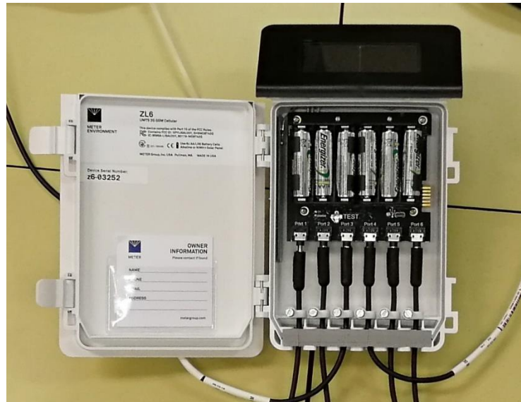
Figure 15. The ZL6 datalogger: a) enclosure; b) Six TEROS 12 sensors connected
