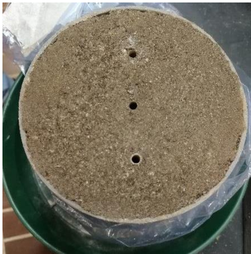
Figure C2. Preparation of the mortar specimens: a) mixing, b) Proctor compaction, c) specimen compacted, d) creation of the needles allocations, e) specimen ready for the installation of the sensor, f) installation of the sensor
