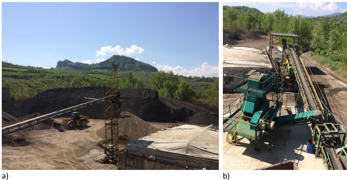
Figure 8. CRM production plant: a) stockpiled RA, b) aggregate selection process
