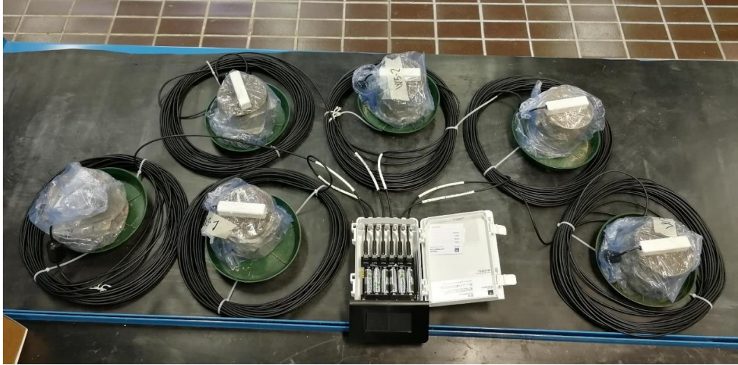
Figure C3. Measurement of the VWC and temperature of the laboratory mortar specimens
