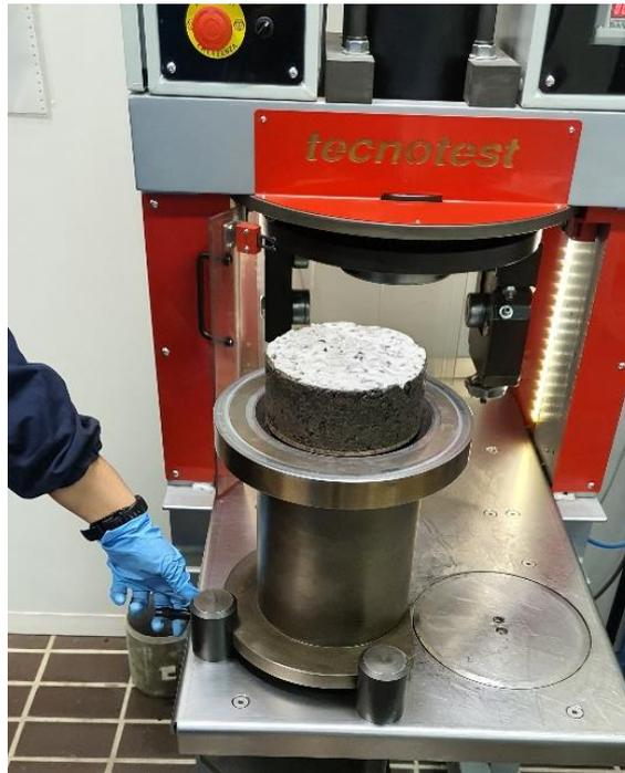
Figure 10. Extrusion of the gyratory compactor specimen
