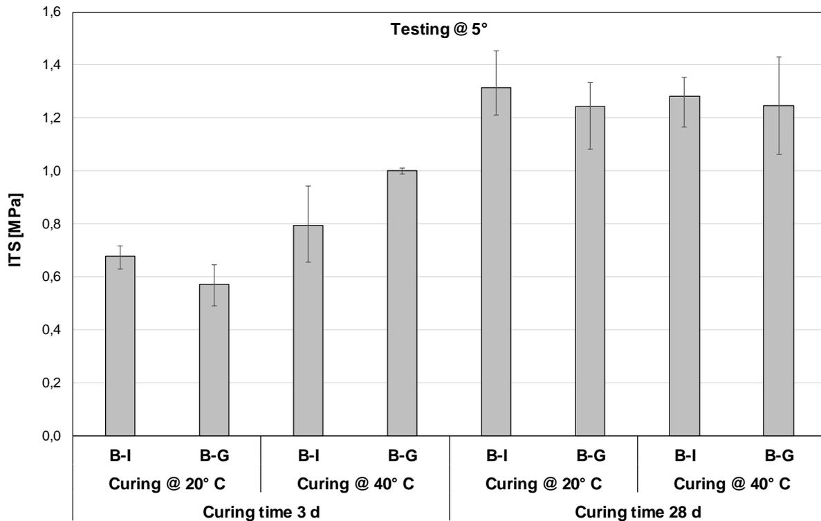
Figure 26. Indirect tensile strength test results obtained for mixture B in usage of Italian (B-I) and German (B-G) bitumen emulsion at test temperature of 5° C
