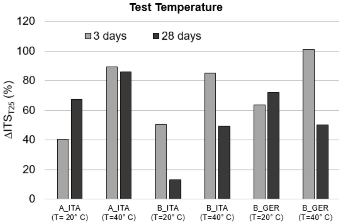
Figure 40. ITS-ratio ( $\Delta ITS_{T25}$ ) of indirect tensile strength considering test temperature for Mix A and mix B
