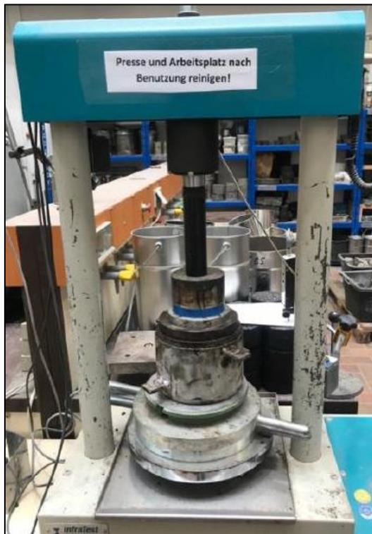
Figure 12. Set up for static compaction at Uni Kassel (left) and University Gustave Eiffel (right)
