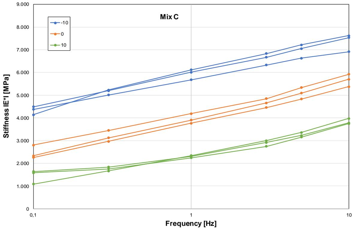
Figure 31. Stiffness of Mix C depending on frequency and temperature
