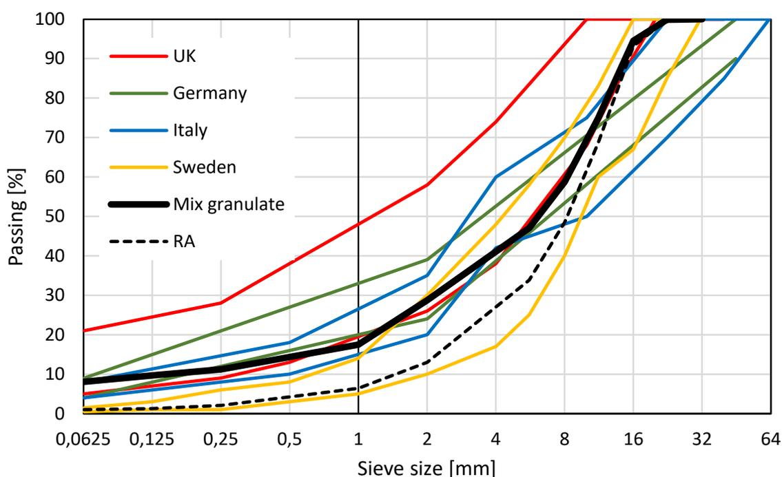
Figure 6. Grading of RA grains and designed mix granulate with added filler and 0/2 aggregates compared to the national specification envelopes
