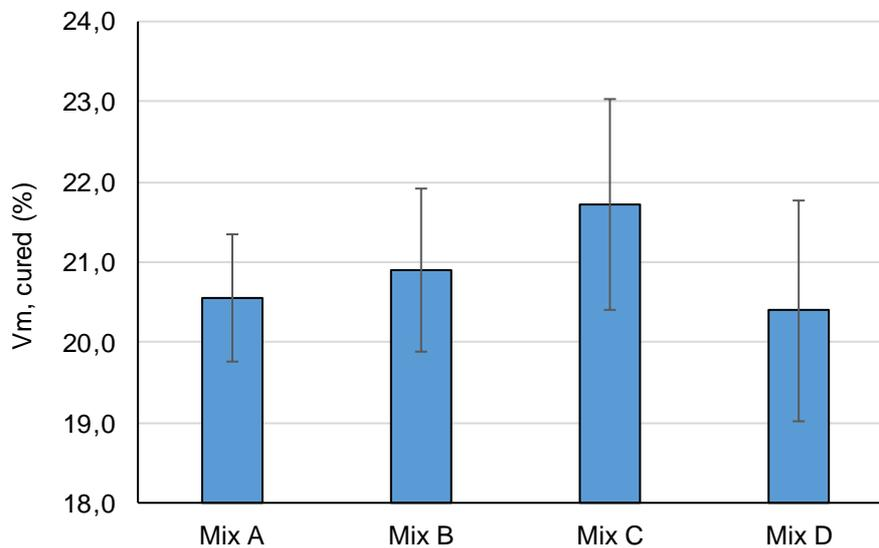
Figure 20. Voids in the mixture A to D (vibratory compaction) at the cured state after 28 days by 20° C
