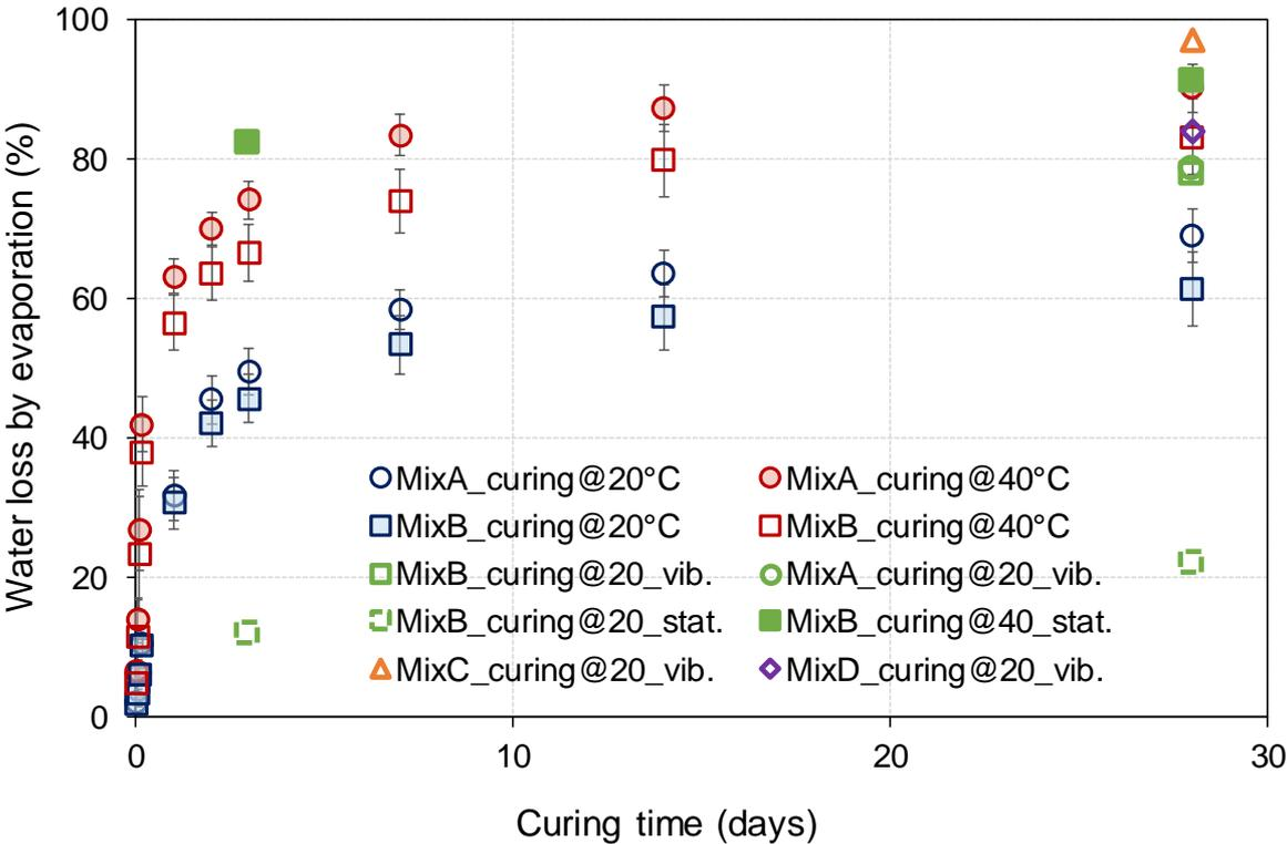
Figure 15. Evolution of water loss by evaporation with curing time
