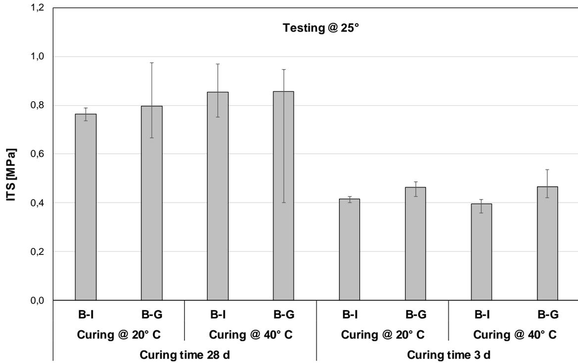
Figure 25. Indirect tensile strength test results obtained for mixture B in usage of Italian (B-I) and German (B-G) bitumen emulsion at test temperature of 25° C
