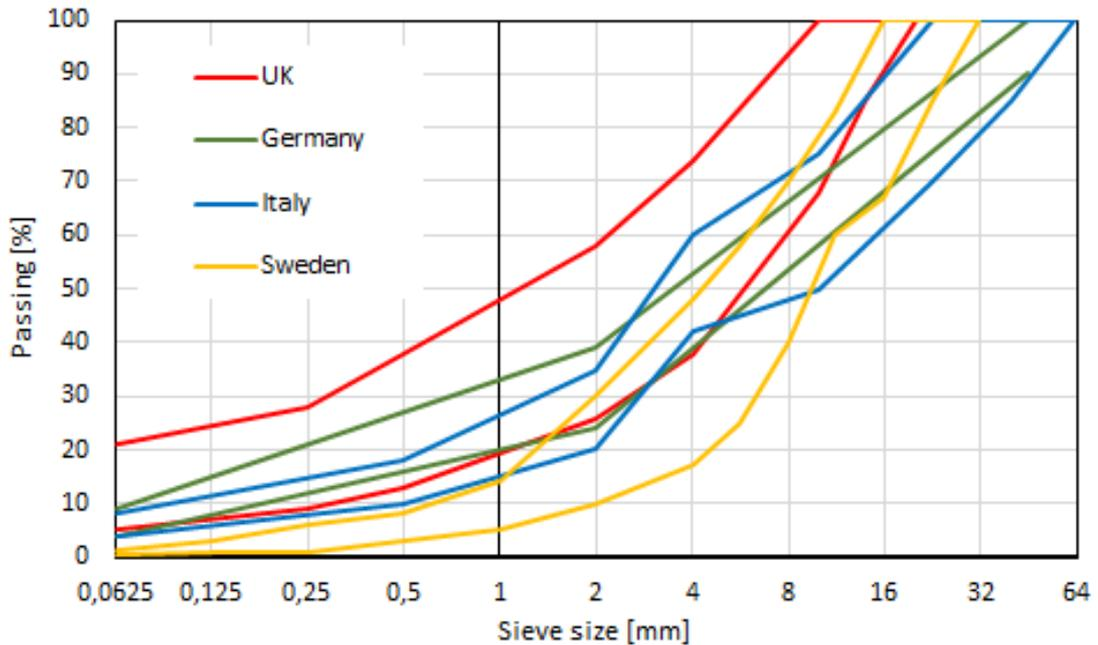
Figure 5. Grading envelopes for mix granulates for cold recycled materials according to four national mix design specifications
