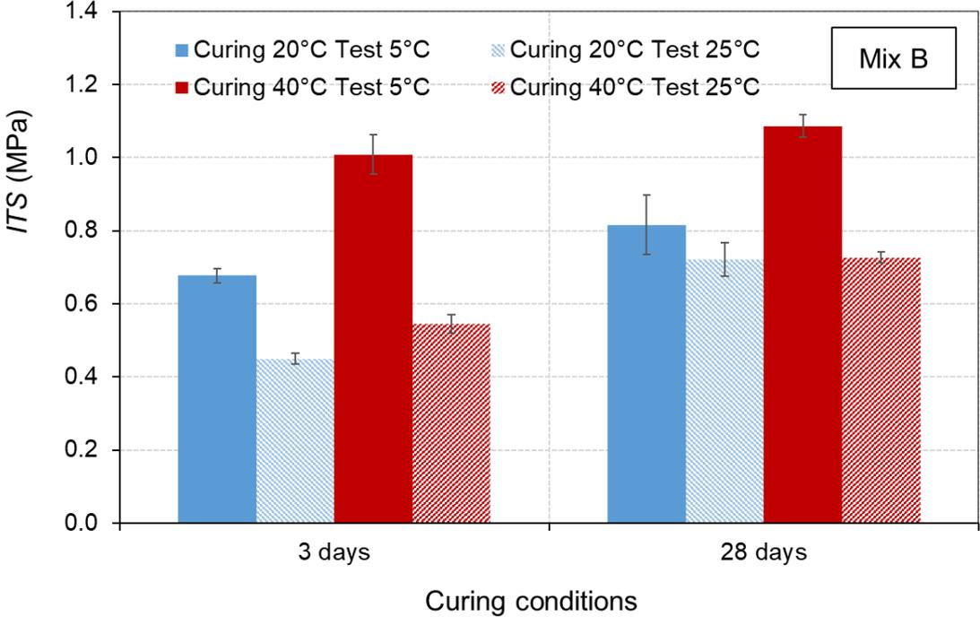
Figure 22. Indirect tensile strength test results obtained for mix B in Italy
