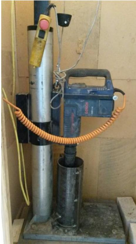
Figure 11. Used vibratory compactor
