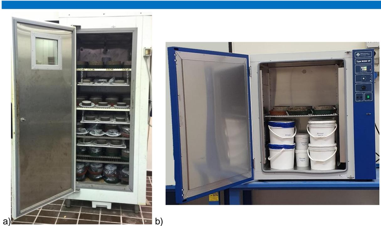
Figure 13. Curing of CRM specimens (ITA) a) climate chamber, b) oven
