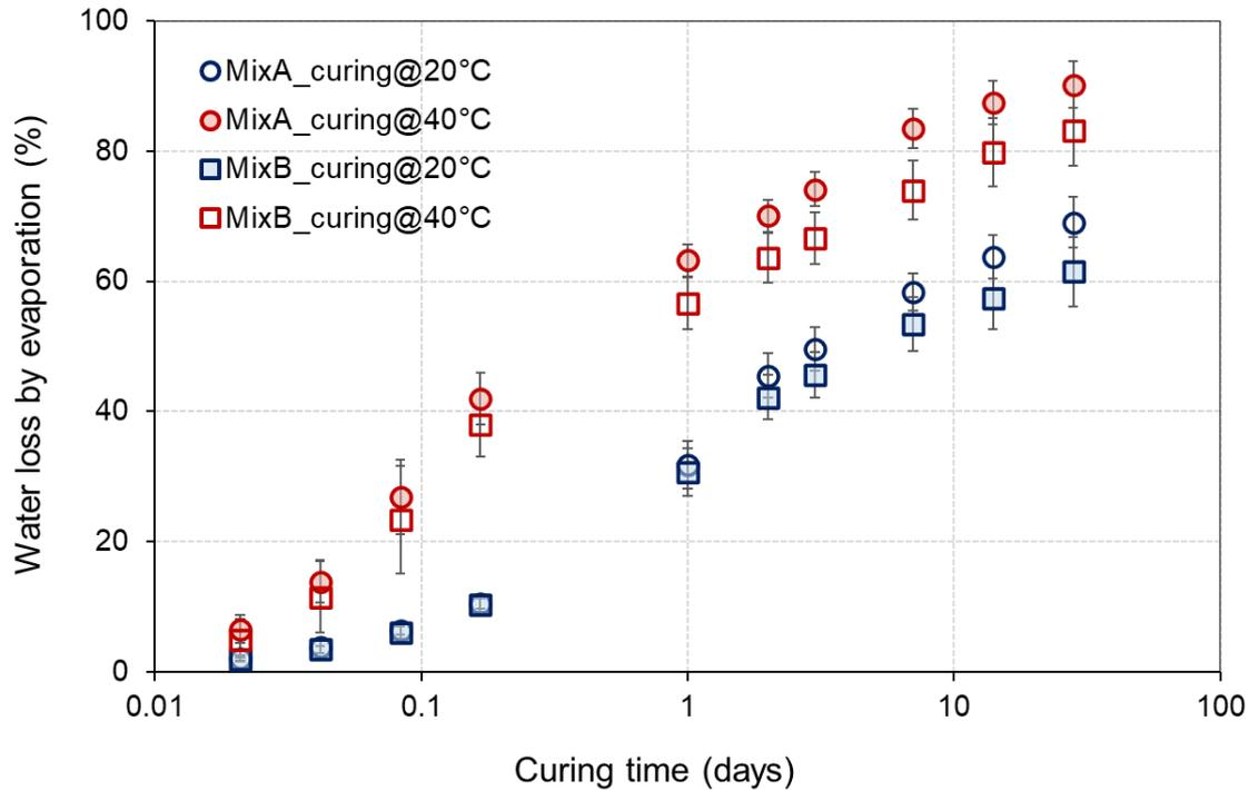
Figure 16. Evolution of water loss by evaporation with curing time (log scale)
