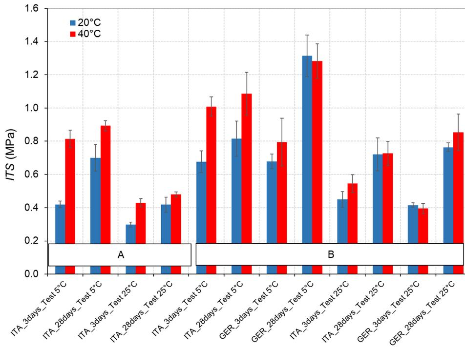
Figure 35. ITS tests results obtained on mixtures A and B changing the curing temperature.
