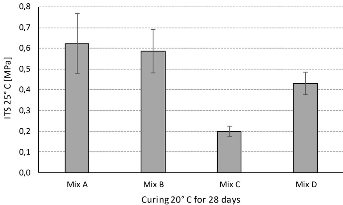
Figure 24. Indirect tensile strength test results obtained for all mixtures in Germany (vibratory compaction)
