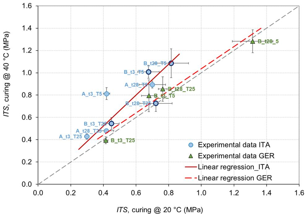
Figure 36. Effect of curing temperature
