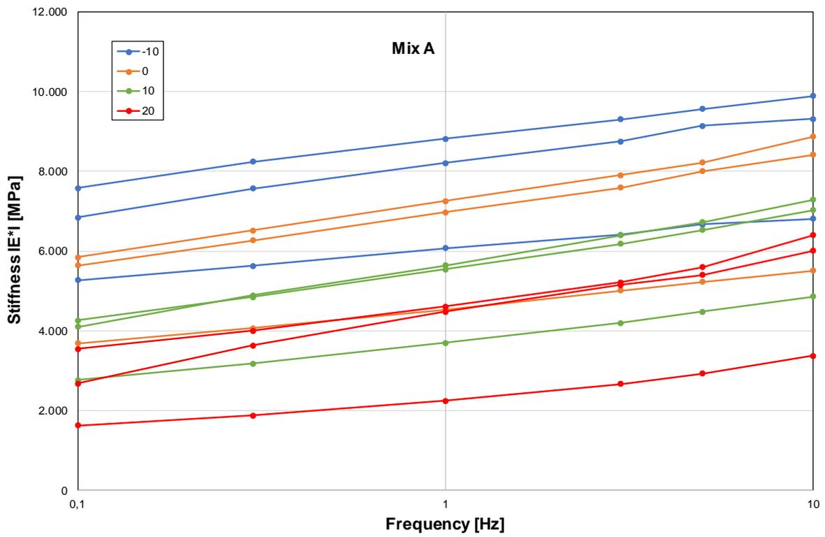
Figure 29. Stiffness of Mix A depending on frequency and temperature
