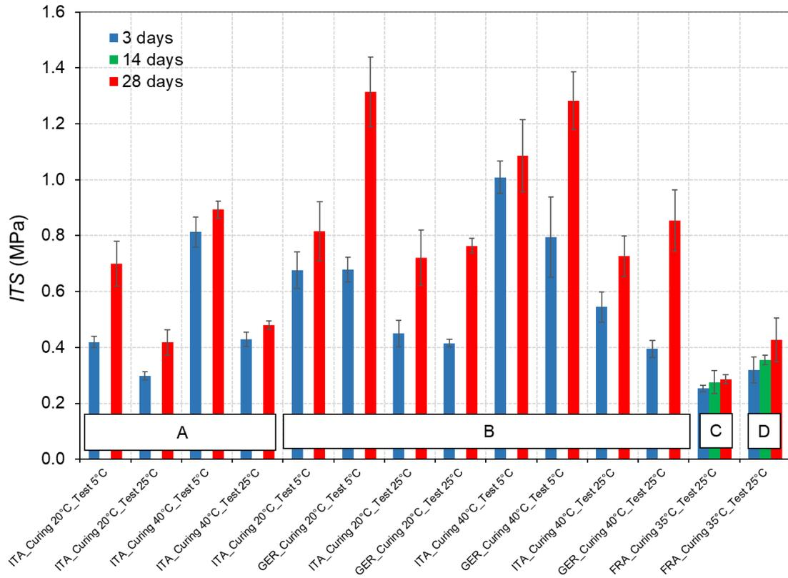
Figure 37. ITS tests results obtained at different curing times
