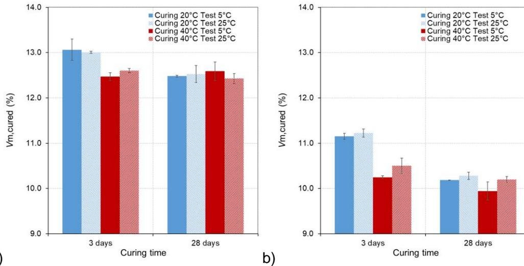
Figure 18. Voids in the mixture at the cured state as a function of curing time (and cement hydration degree) a) mixture A, b) mixture B
