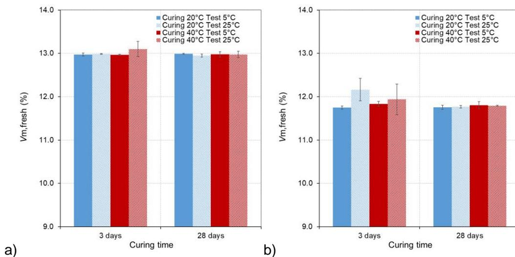
Figure 17. Voids in the mixture at the fresh state a) mixture A, b) mixture B
