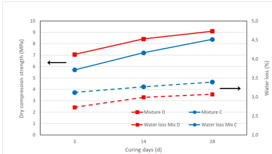
Figure 27. Dry compressive strength test results obtained for mixtures C and D in France at test temperature of 18° C
