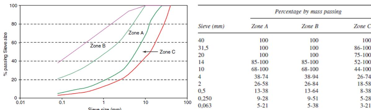
Figure 1. Grading curves for cold recycled mixtures and particle size distribution of mixture for cold recycling adapted from UK mix design specifications
