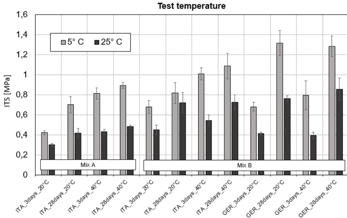
Figure 39. Indirect tensile strength test results obtained for Mix A and B
