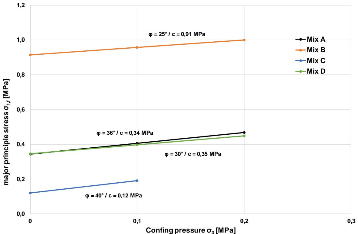
Figure 28. Shear strength test results obtained for all mixtures in Germany
