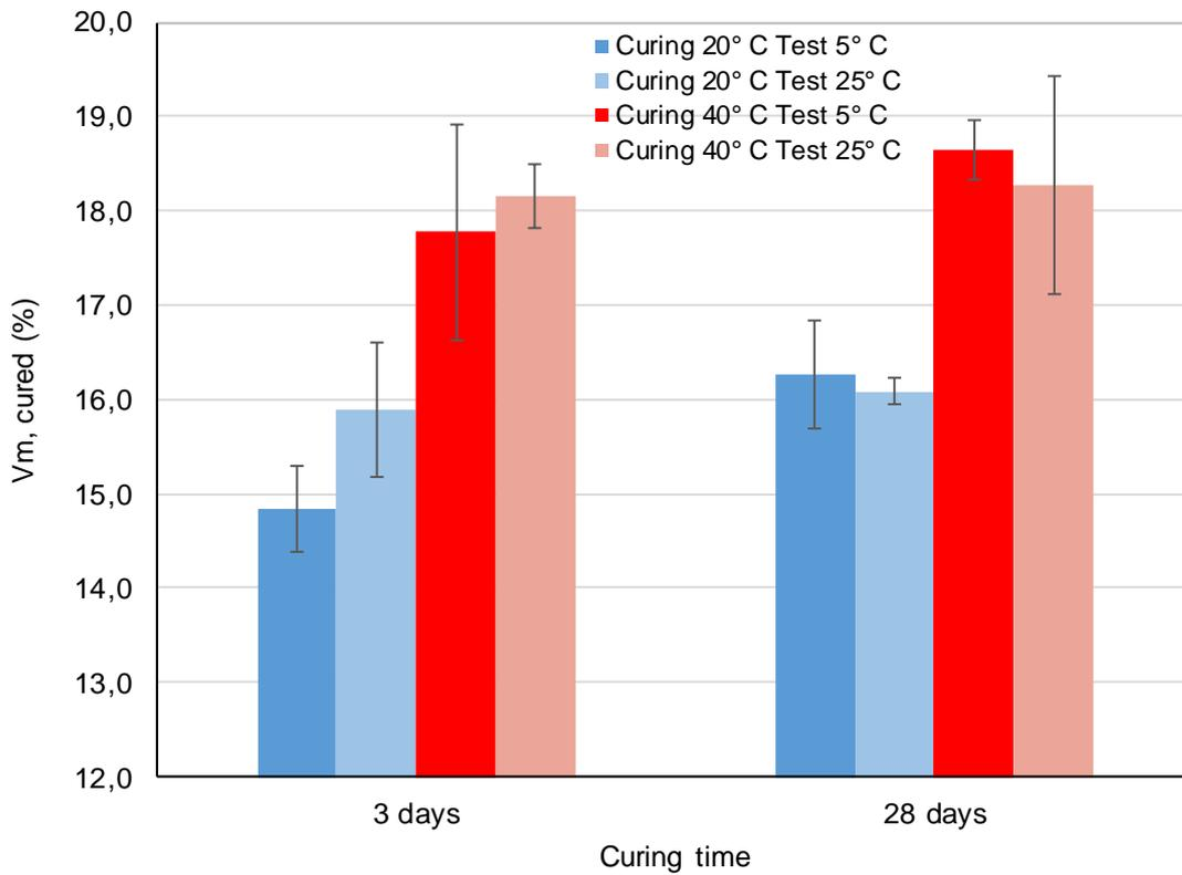
Figure 19. Voids in the mixture at the cured state as a function of curing time mixture B (static compaction)
