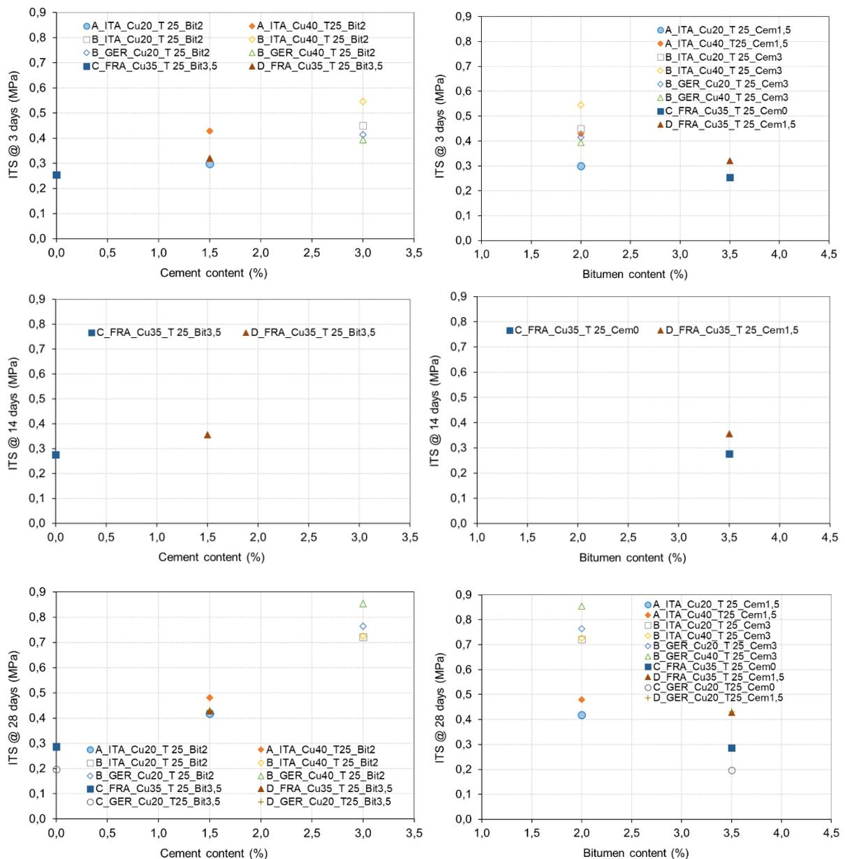
Figure 34. ITS tests results obtained at 25 °C on mixtures A to D, plotted versus cement content (left) and bitumen content (right).
