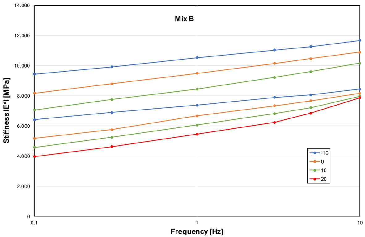
Figure 30. Stiffness of Mix B depending on frequency and temperature
