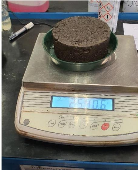
Figure 14. Weighing of the CRM specimen before the start of the curing (ITA)
