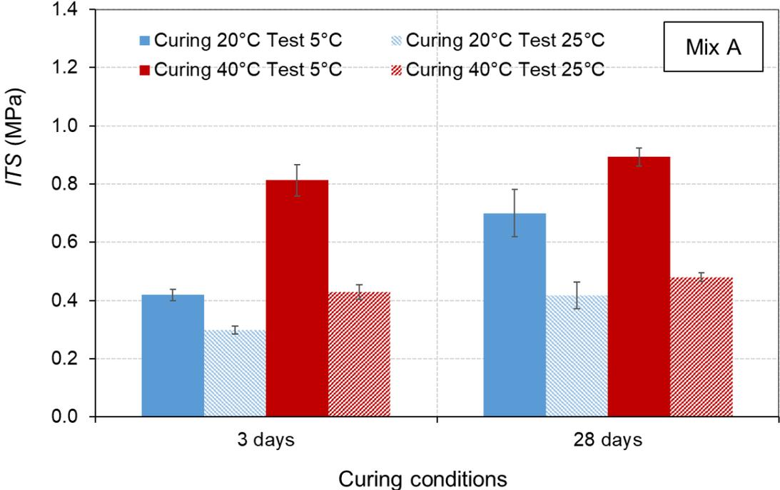
Figure 21. Indirect tensile strength test results obtained for mix A in Italy
