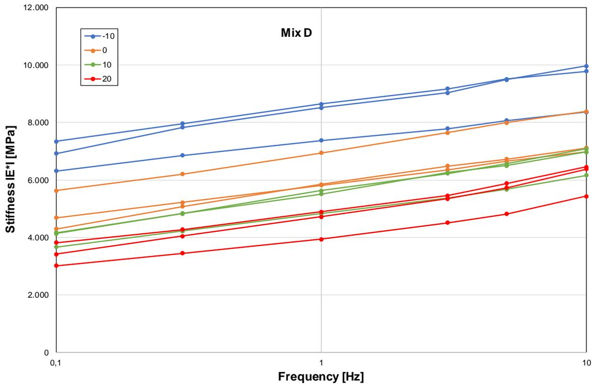
Figure 32. Stiffness of Mix D depending on frequency and temperature
