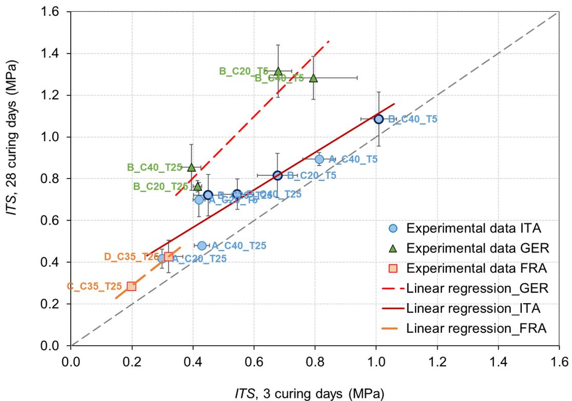
Figure 38. Effect of curing time
