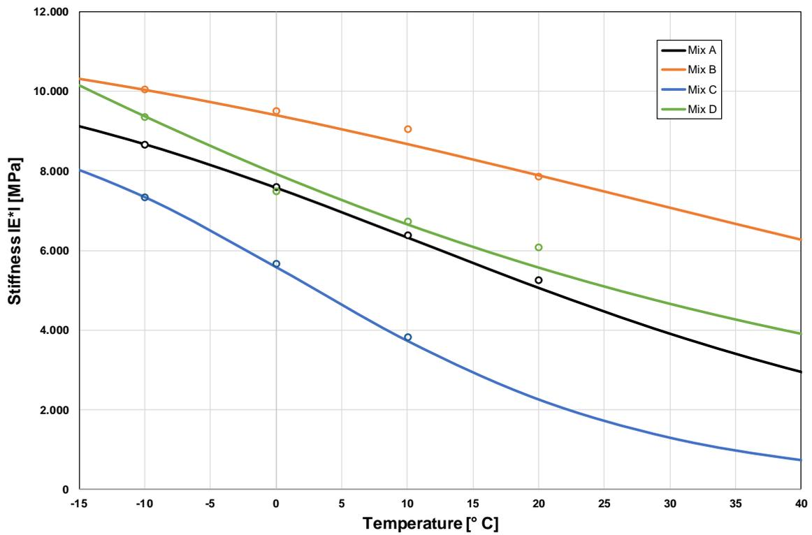
Figure 33. Stiffness-temperature-function calculated for Mix A to D
