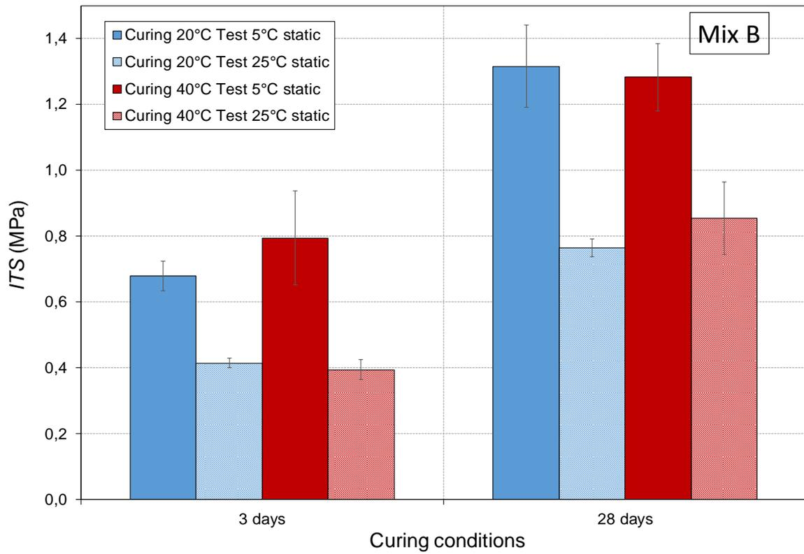
Figure 23. Indirect tensile strength test results obtained for mix B in Germany
