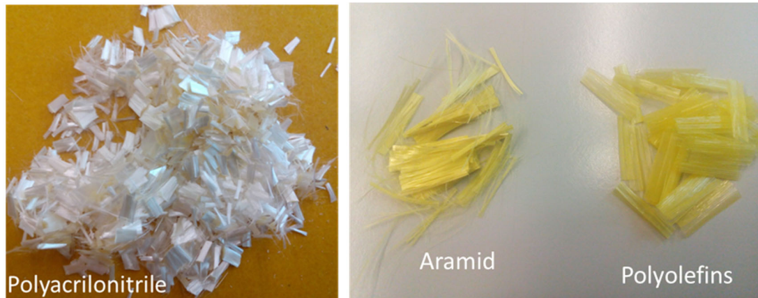
Figure 3. Selected fibres from WP2 study. Left: Polyacrylonitrile. Right: blend aramid/polyolefin
