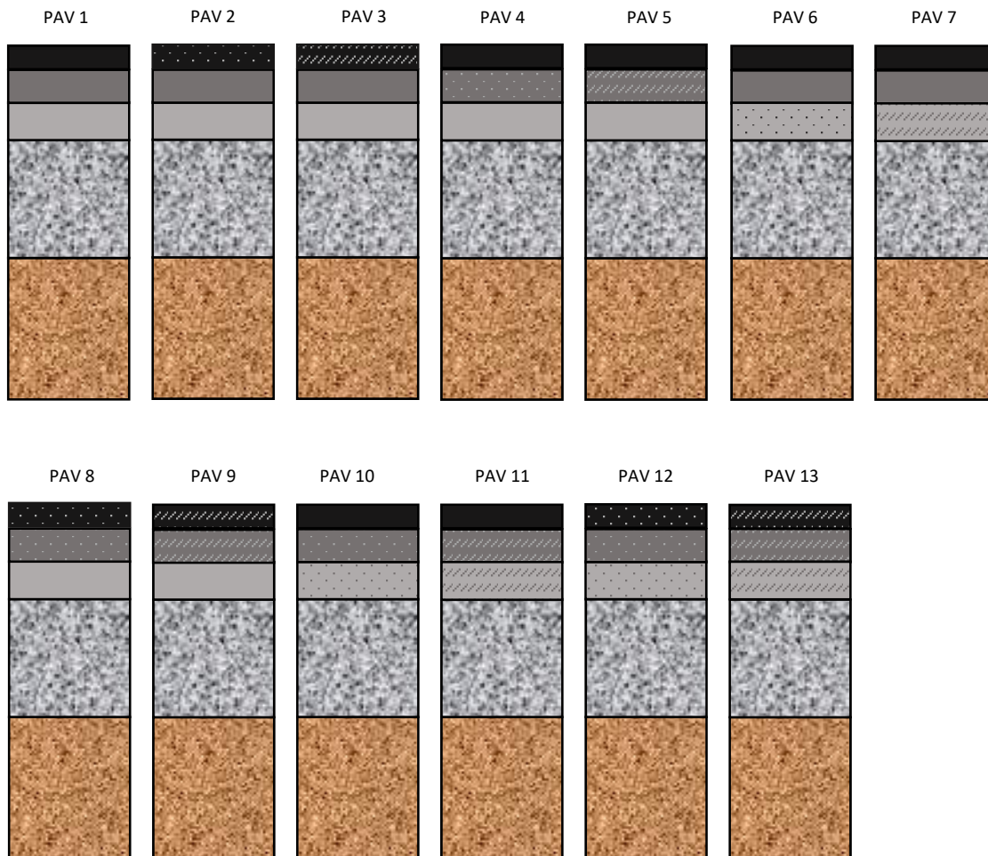
Figure 10. Pavement sections simulated with FlexPAVE™. See fig 11 for definitions of grey scale
