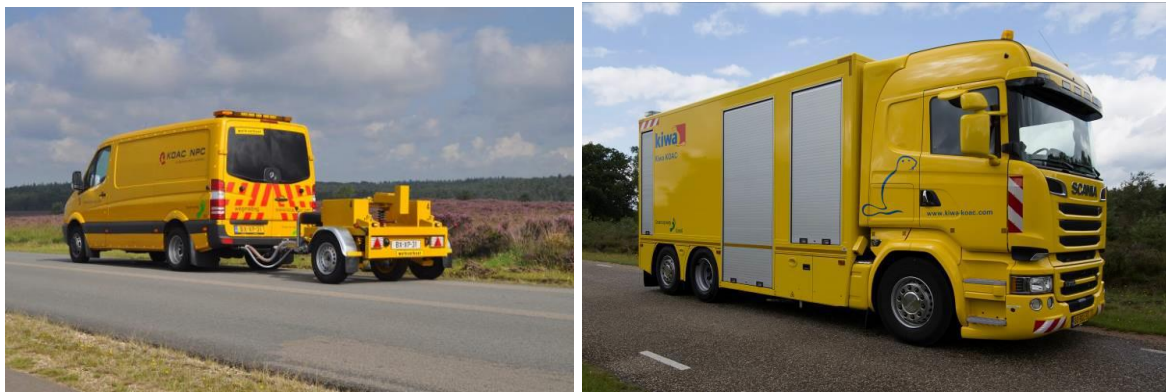
Figure 24. Illustration of measurement of skid resistance by the use of RAW 2015/72 (left) and side way force (right)
