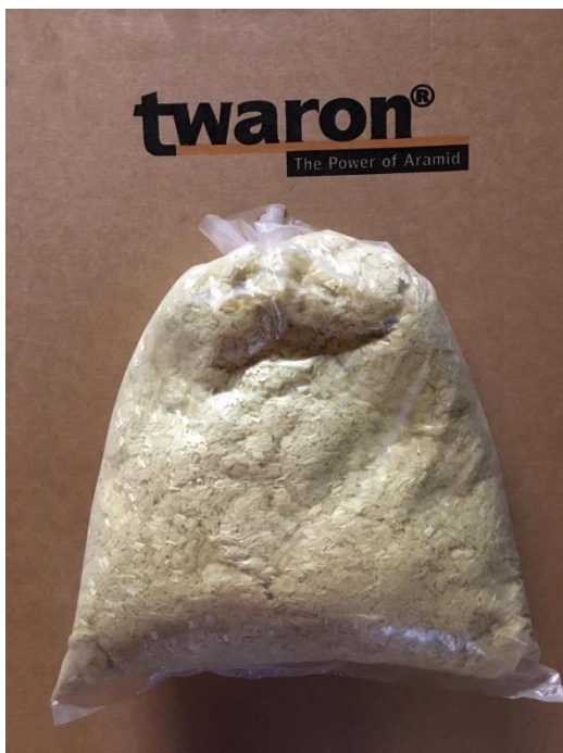
Figure 8. Example of aramid fibres in low-melt bag (left) and the inspection opening of the mixer (right) used to manually insert the bags into the mixer.
