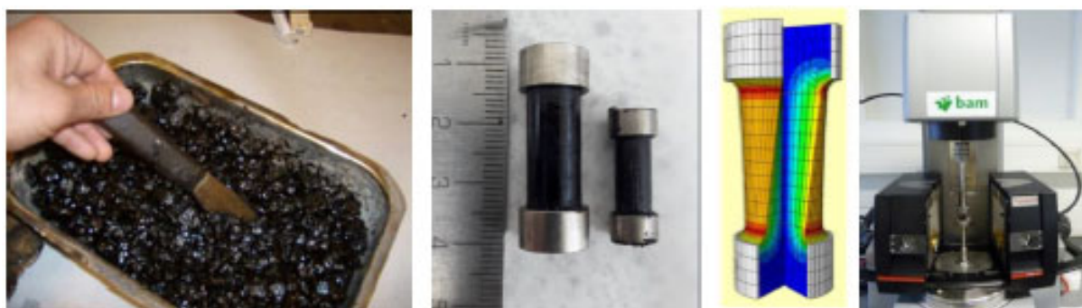
Figure 7. DSR mortar response test of hopper materials on A73 test sections
