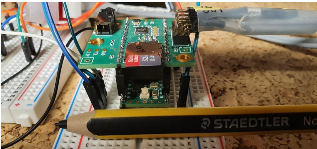
Figure 6: Assembling the on-board system Teensy 4.0 and its audio adaptor.
