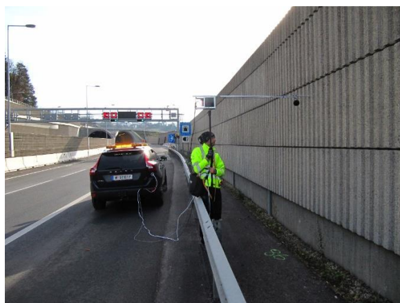
Figure 5: portable device for measuring sound reflection [©AIT, unpublished]
