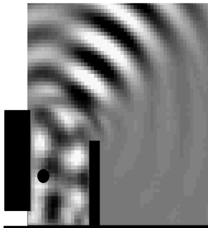
Figure 16: Propagation of continuous waves on a reflecting obstacle: interactions with a truck body (black rectangle on the left) [3]
