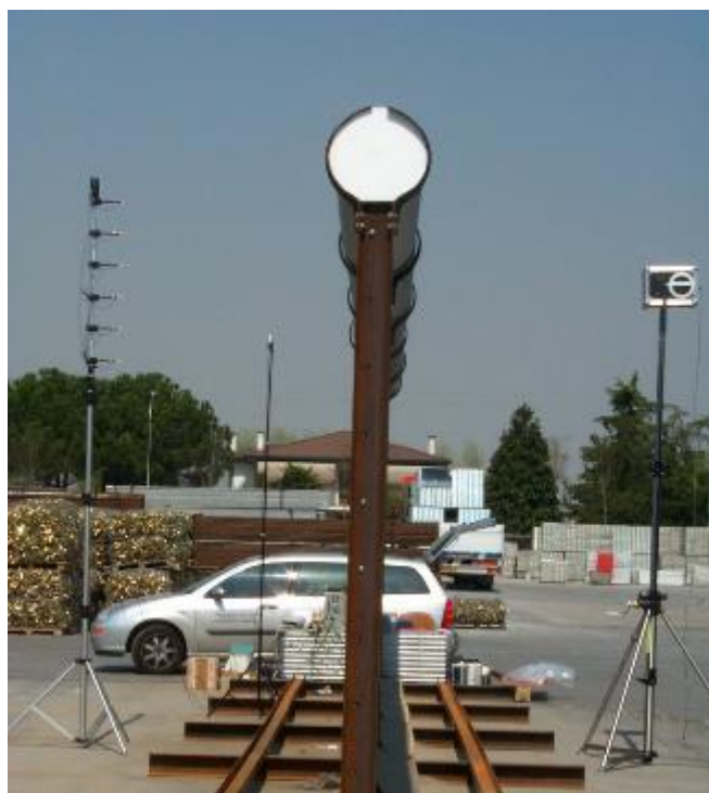
Figure 53: Sound diffraction index measurements according to EN 1793-4 on a prototype added device
