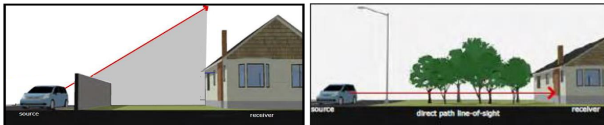
Figure 1: To reduce traffic noise, NB are placed as obstacles to the sound propagation [1]
