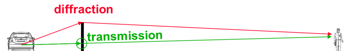
Figure 27: Noise behind the NB = transmitted noise + diffracted noise
