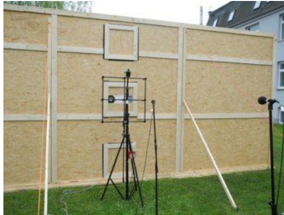
Figure 14: Noise barrier test stand with defined and variable slit and hole size; used for the validation of the theoretical model developed by Mechel. ©BASt
