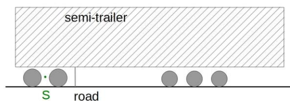
Figure 44: Position of the assumed point source “S” near the traction wheels of the dolly beneath a semi-trailer
