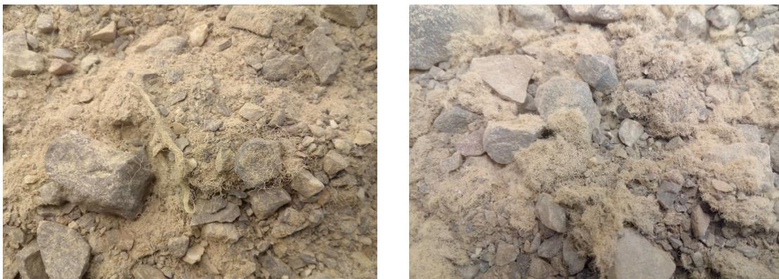
**Figure 10. Mineral aggregates and fibres after bitumen extraction. FRAMs modified with fibres type A (left) and type P (right).**
