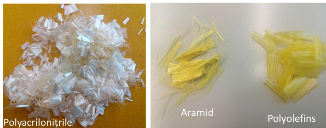
Figure 1. Images of the different fibres used for the WP3. Type P (left) and type A (right).
