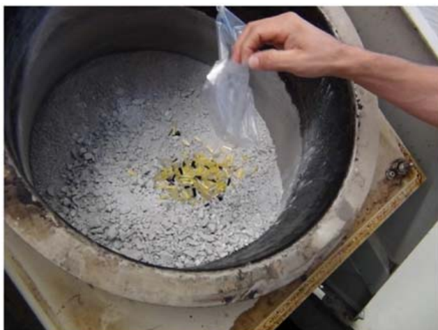
Figure 9. Addition of fibers to the hot aggregates, before asphalt binder addition. (Klinsky et al., 2018)
