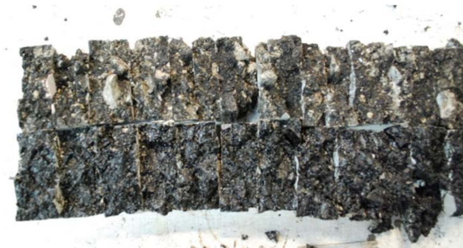
Figure 28. Binder coverage seems to be better in the reference section (conventional HMA), shown in the bottom row compared to the CRM layer shown in the top row.
