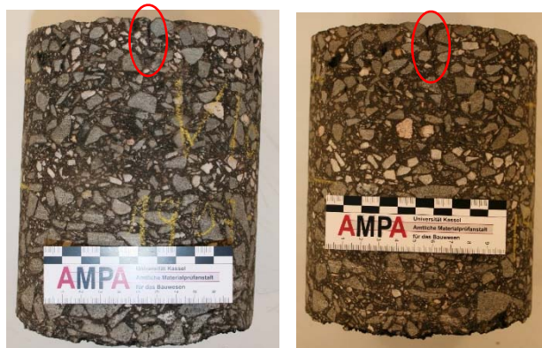
Figure 9. L386 cores extracted from cracked zones.
