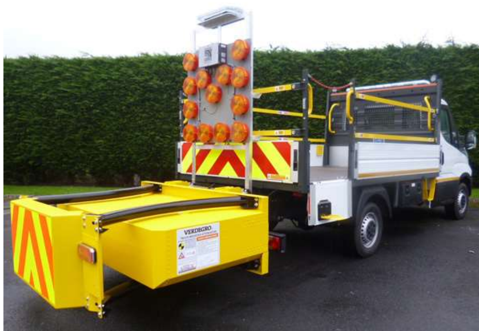
Figure 29. TMA, equipped with crash cushion and various LEDs (beacon bars, work lights, strobes). Source: www.roadsafety.co.uk
