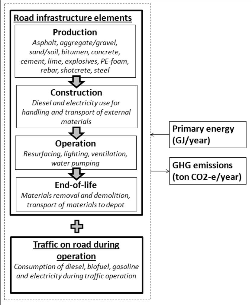
Figure 1: Simplified system boundaries in the LICCER model
