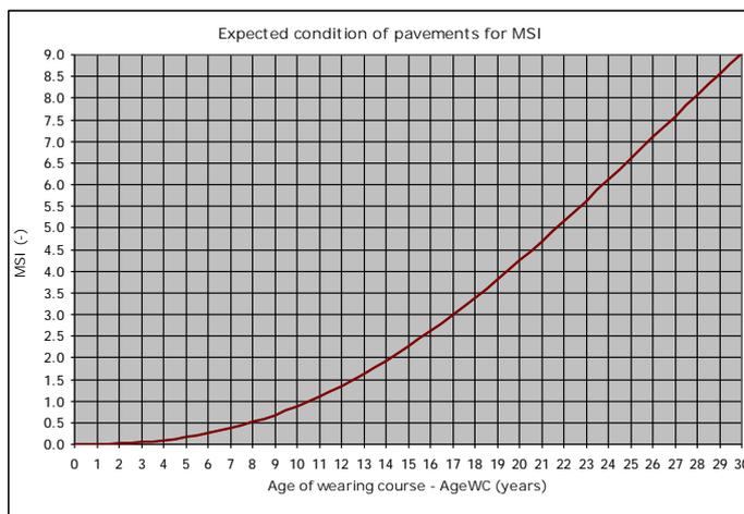
Figure 5: Expected condition of pavement, expressed with MSI
