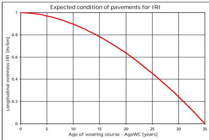
Figure 10 Normalized expected condition of pavement, expressed with IRI
