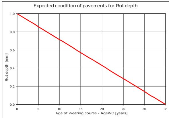
Figure 8 Normalized expected condition of pavement, expressed with Rut depth (mm)
