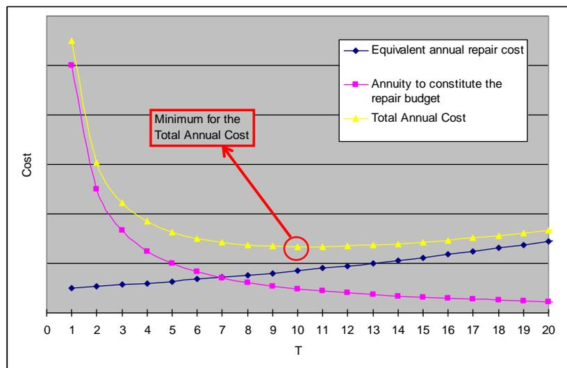
Figure 13 The evolution of the annually discounted repair and maintenance costs
