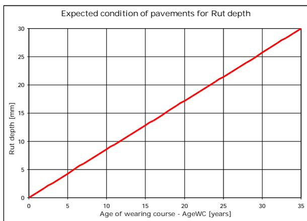
Figure 7 Expected condition of pavement, expressed with Rut depth (mm)
