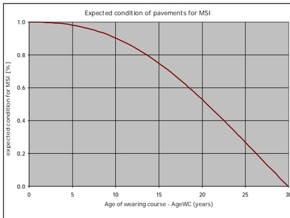
Figure 6 Normalized expected condition of pavement, expressed with MSI
