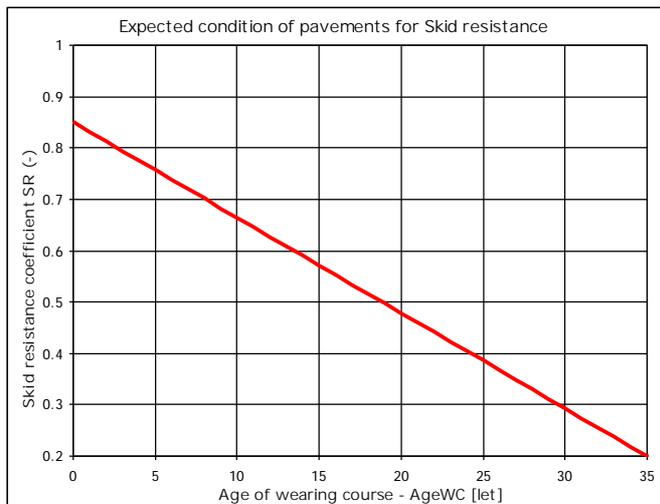
Figure 11 Expected condition of pavement, expressed with Skid resistance coefficient SR (-)
