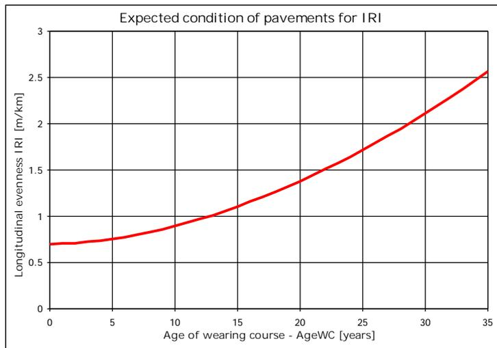
Figure 9 Expected condition of pavement, expressed with IRI
