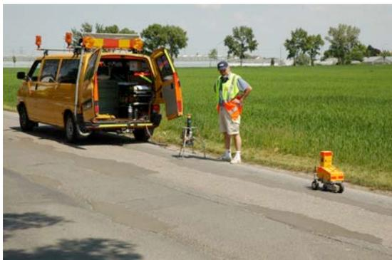
Figure 1 Longitudinal evenness – VTI primal, VTI, Sweden (SPENS 2008)
