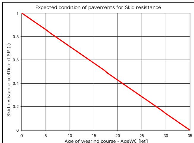
Figure 12 Normalized expected condition of pavement, expressed with Skid resistance coefficient SR (-)
