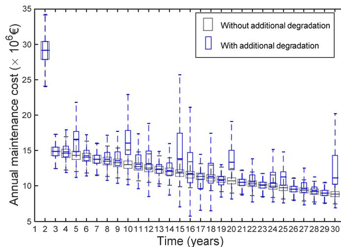
**Figure 26. Annual maintenance cost for structural components without or with additional degradation due to climate change.**
