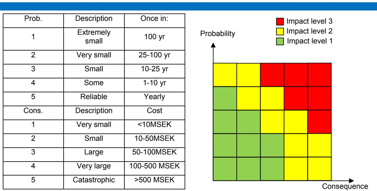
**Figure 4. Risk matrix used to sort the climate change-induced events according to their level of impact (NVF, working group 41. 2008-03-25, working material).**
