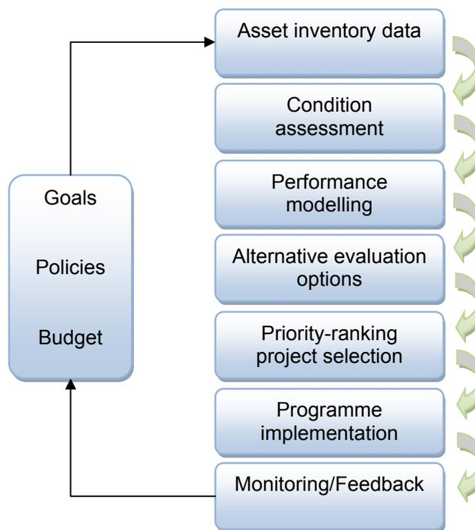
**Figure 3. Components of an asset management (PIARC 2004b).**
