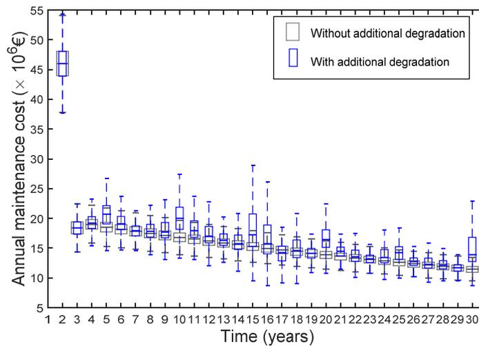
**Figure 25. Overall annual maintenance cost without or with additional degradation due to climate change.**
