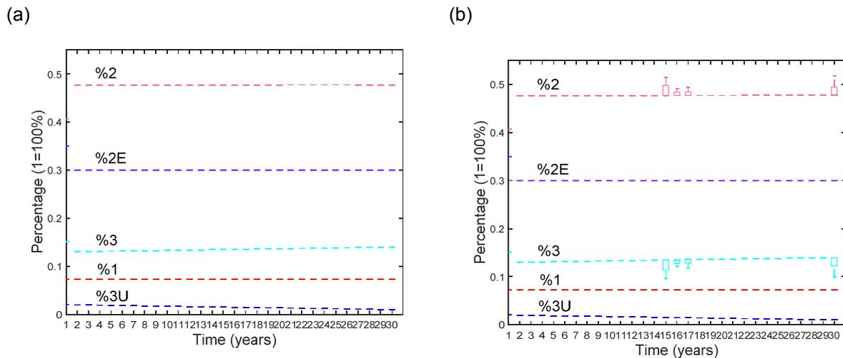
**Figure 28. Percentage in each condition score for structural components (a) without and (b) with additional degradation due to climate change.**
