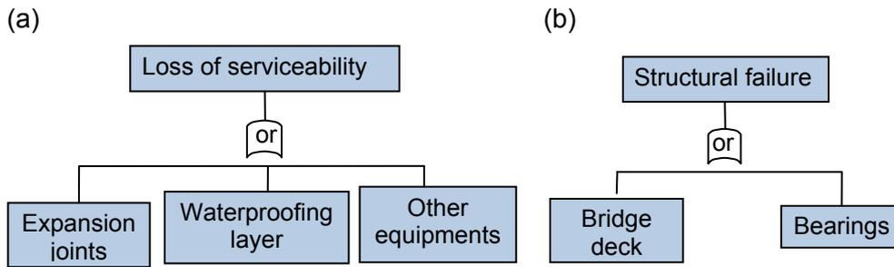
**Figure 12. Fault tree model used for bridges (French case study) (a) loss of serviceability and (b) structural failure.**
