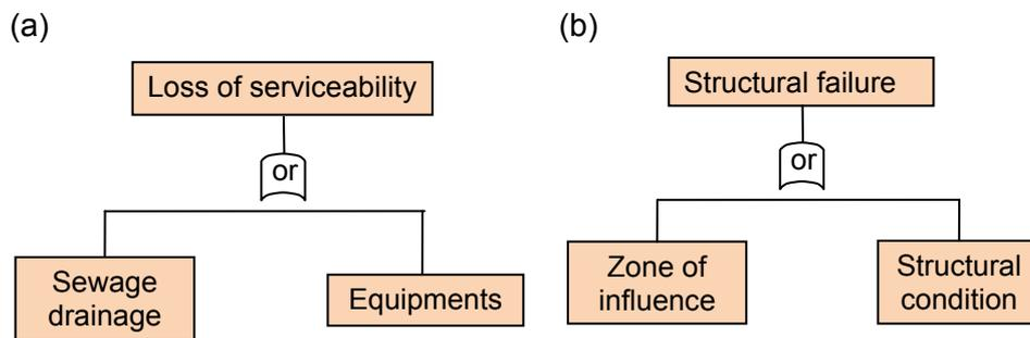
**Figure 13. Fault tree model used for walls (French case study) for (a) loss of serviceability and (b) structural failure.**
