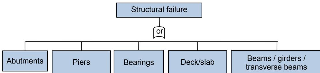
**Figure 6. Fault tree model used for bridges (Irish case study) for (a) loss of serviceability and (b) structural failure.**
