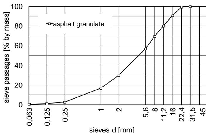
**Figure 20: Grading of particle size for reclaimed asphalt**
