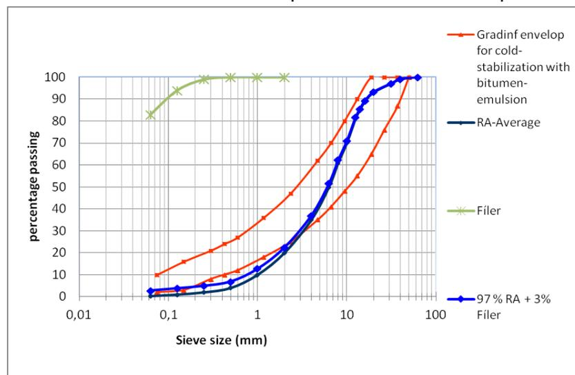
Figure 18: RA, filler and final granulate material grading curves
