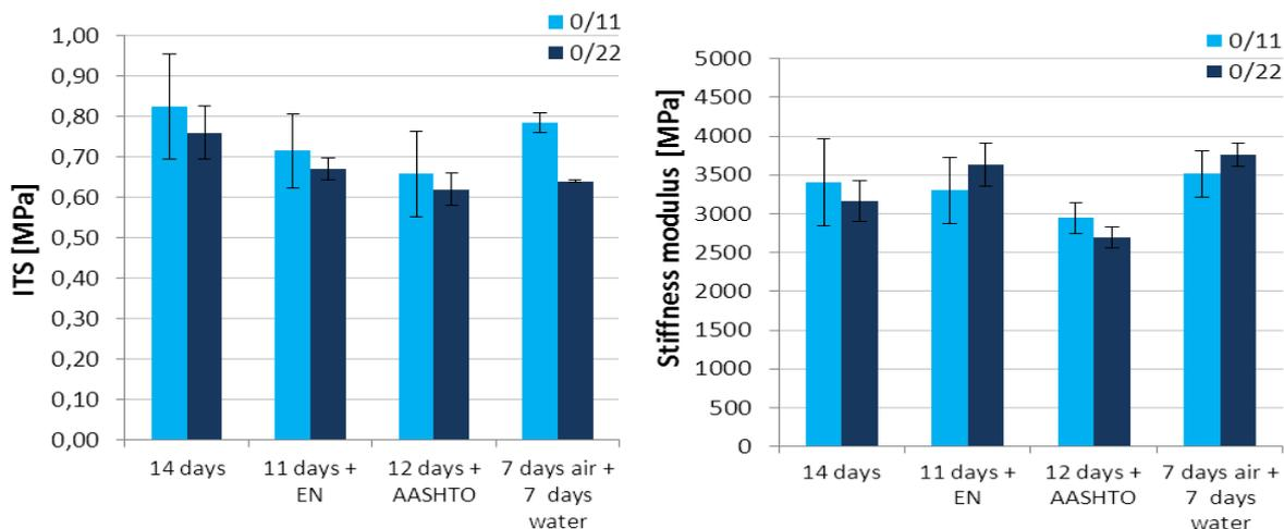
Figure 7 and 8: Determined values of ITS and stiffness modulus – mix B
