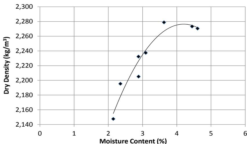
Figure 16: Determination of Optimum Moisture Content
