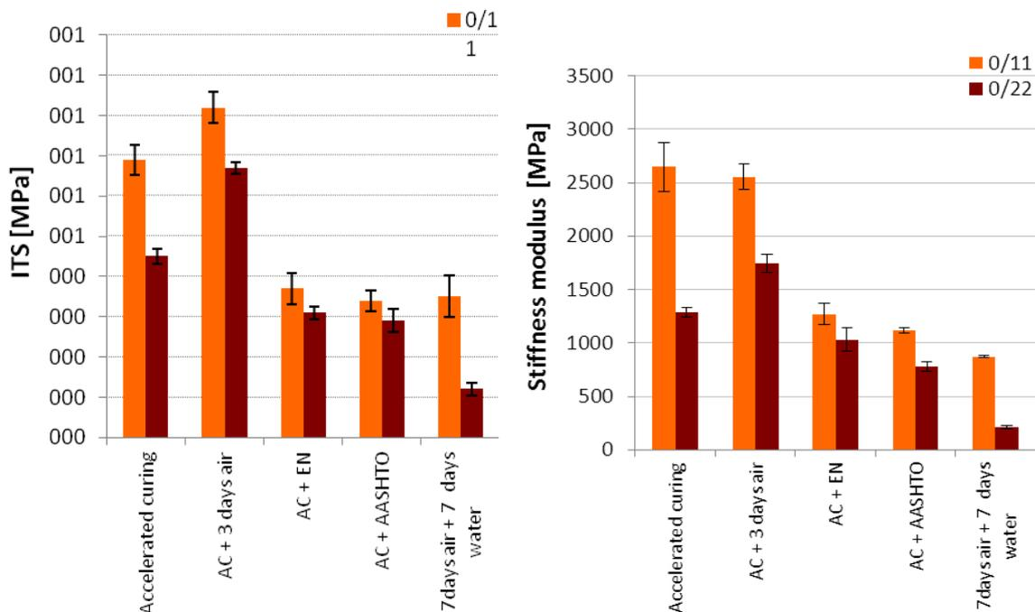
**Figure 1 and 2: Determined values of ITS and Stiffness modulus – mix C**
