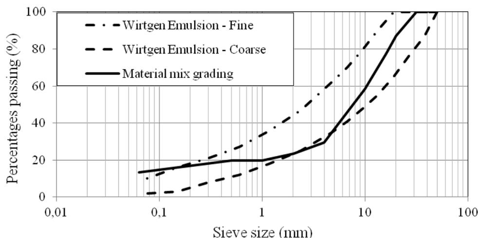
Figure 15: Material Mix Grading
