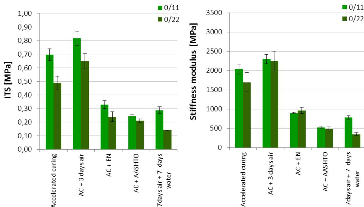
**Figure 3 and 4: Determined values of ITS and Stiffness modulus – mix D**
