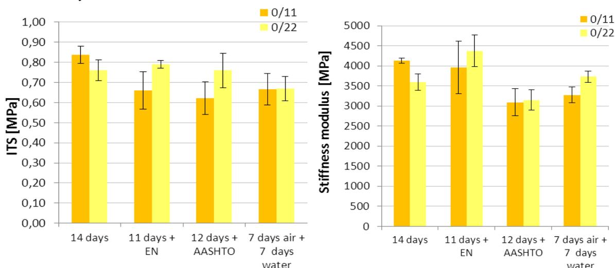
**Figure 5 and 6: Determined values of ITS and Stiffness modulus – mix A**
