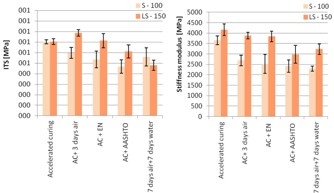
Figure 11 and 12: Determined values of ITS and stiffness modulus – mix S
