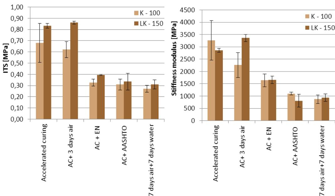
Figure 9 and 10: Determined values of ITS and stiffness modulus – mix K
