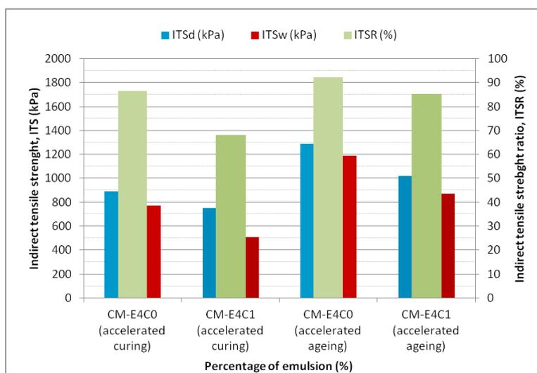
**Figure 19: Water sensitivity of cold recycled mixes aged or not**
