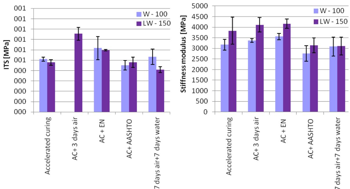
Figure 13 and 14: Determined values of ITS and stiffness modulus – mix W
