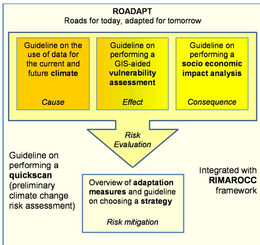
Figure 3.2: Structure of the ROADAPT guidelines
