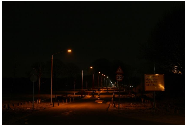
Figure 3-11 Amber coloured street lighting may minimise the light disturbance of a bat flight path. Furthermore, the lamps on this path in the Netherlands are controlled by motion sensors, and only switch on when there are bicycles or pedestrians on the road. Photograph by V. Loehr.
