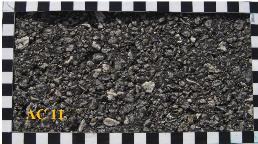
Figure 4.10: Close up photo of a SMA16 pavement normally used as a reference in Sweden (top) and a dense asphalt concrete with 11 mm aggregates (AC 11) used as a reference in Nord2000 in Denmark (bottom). The size of the black and white squares is 10 x 10 mm.
