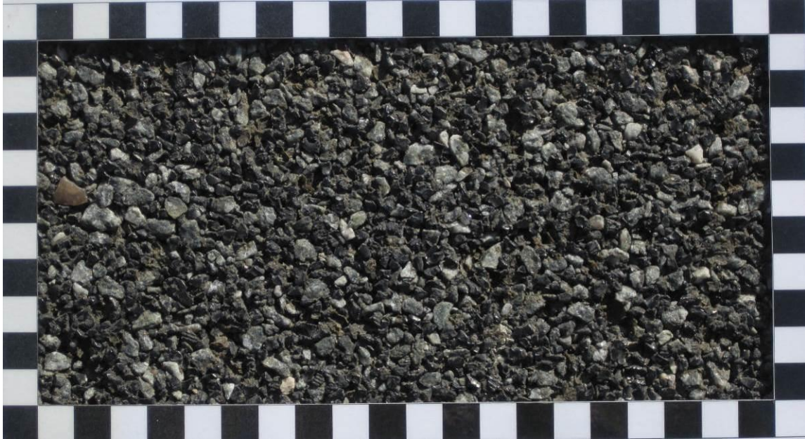
Figure 5.14: Close-up photo of ten month old poroelastic pavement on test section at Kalvehave in Denmark. The size of the black and white squares is 10 x 10 mm. The dark aggregates are rubber and the lights are stone aggregates [14, 27].
