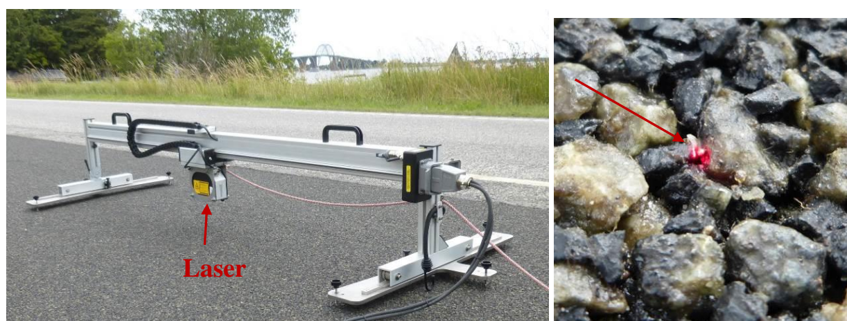
Figure 5.3: Laser equipment for measurement of pavement surface texture (left). The red laser beam can be seen on the pavement (right).
