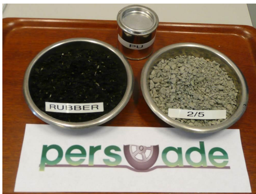
Figure 5.13: The components used in poroelastic pavements are stone aggregates here 2/5 mm maximum aggregate size, granulated rubber from scrapped tyres and polyurethane.
