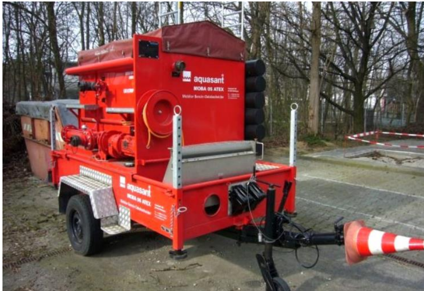
Figure 7: Example of a mobile emulsion/flotation splitter used in Switzerland (photo: Swiss Federal Roads Office)
